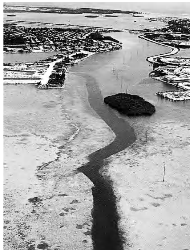
Fig. 8.28 Dredged channels as a waterway to a new marina in weakly cemented coral carbonates at the Florida Keys, USA (left) and the Palau islands of Micronesia (right). (Photo credit: D. Kelletat).
