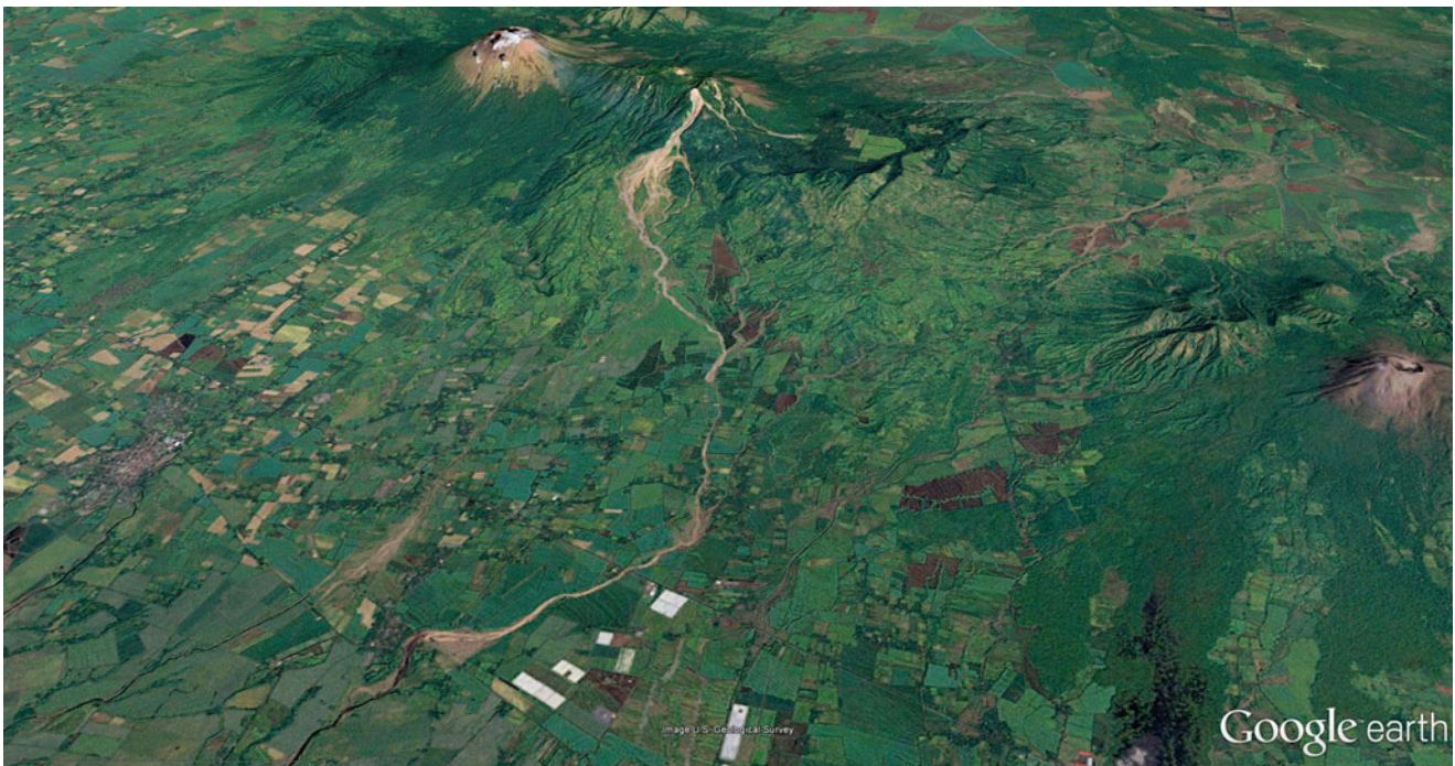
Fig. 8.12 La Casita landslide and lahar pathway in Nicaragua. On October 30th, 1998, hurricane Mitch resulted in intense rainfall in Central America, causing parts of the southern flank of the Casita volcano to slide. The original mass of the slide successively increased by incorporating volcanic material and water and turned into a lahar (from a hyper-concentrated flow and later a debris flow). The La Casita event
