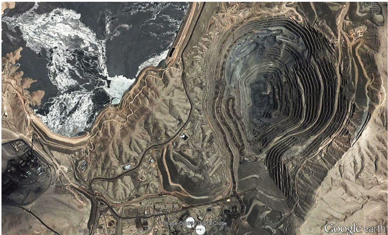
Fig. 14.10 Copper mining in the Chuquicamata Mine (near Copiaco, Chile) at 27^{\circ}31'S and 70^{\circ}18'W . Scene is 7.5 km wide. The maximum depth of the open pit is 1,000 m. It is the largest copper mine of the
