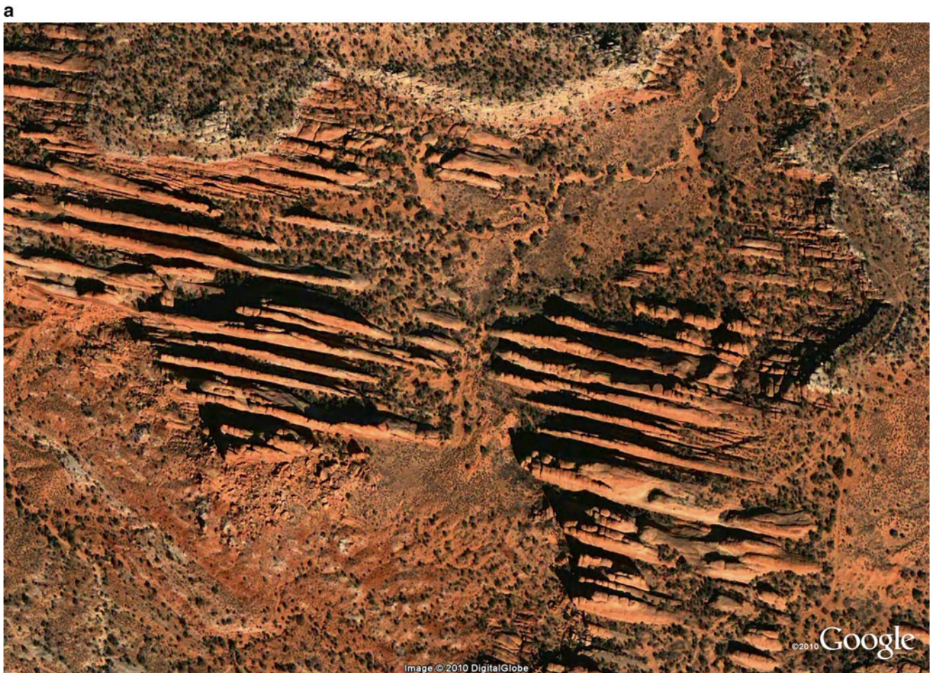
Fig. 4.32 (a) In Arches National Park (Utah, USA), main joints have been weathered to more than 30 m deep leaving behind delicate, fin-like structures. Scene is 3 km wide at 38^{\circ}50'N and 109^{\circ}41'W
