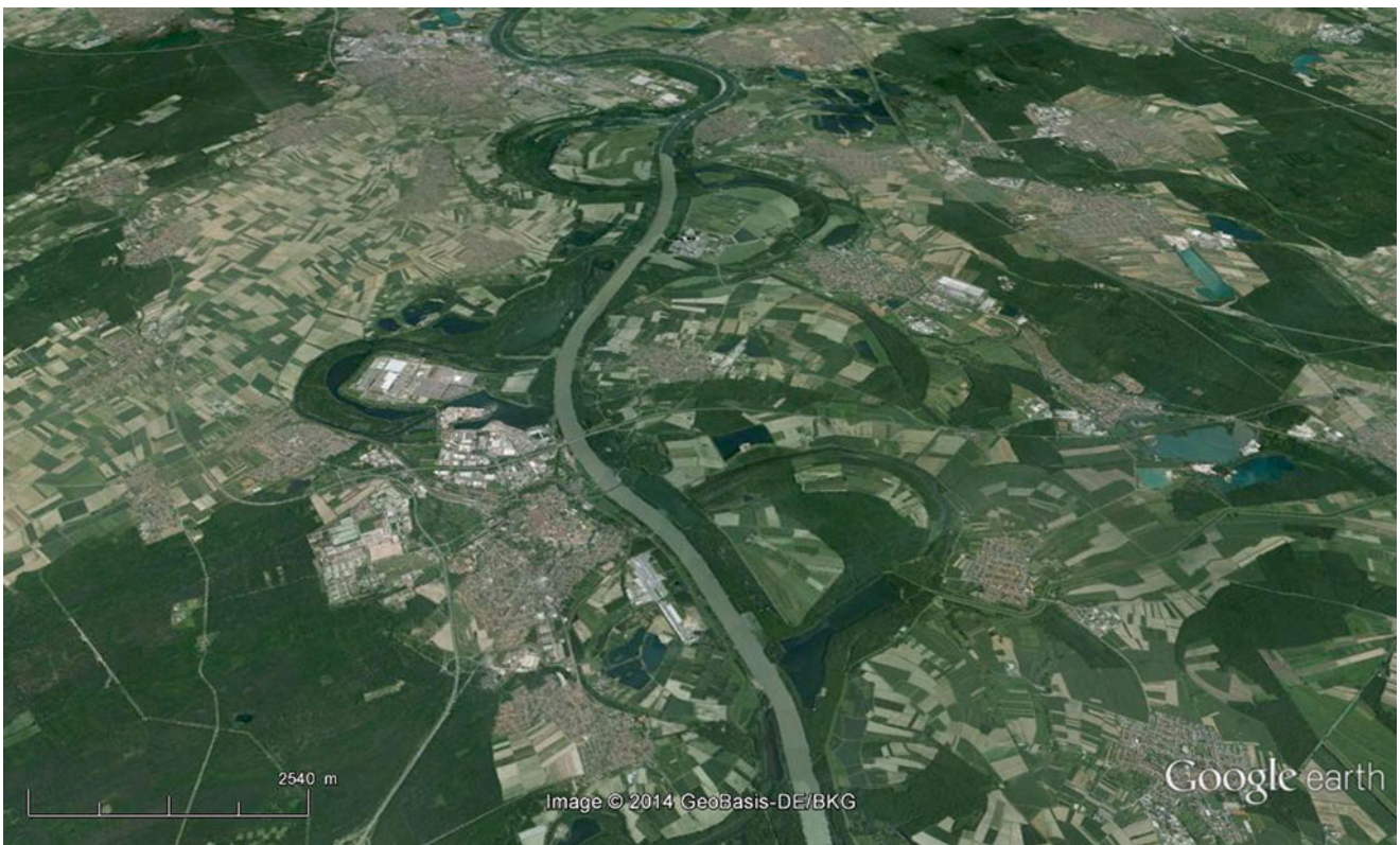
Fig. 14.13 Artificial shortening of a river course for shipping purposes (River Rhine in Germany at 49^{\circ}13'N and 8^{\circ}24'E ) (Image credit: ©Google earth 2012)
