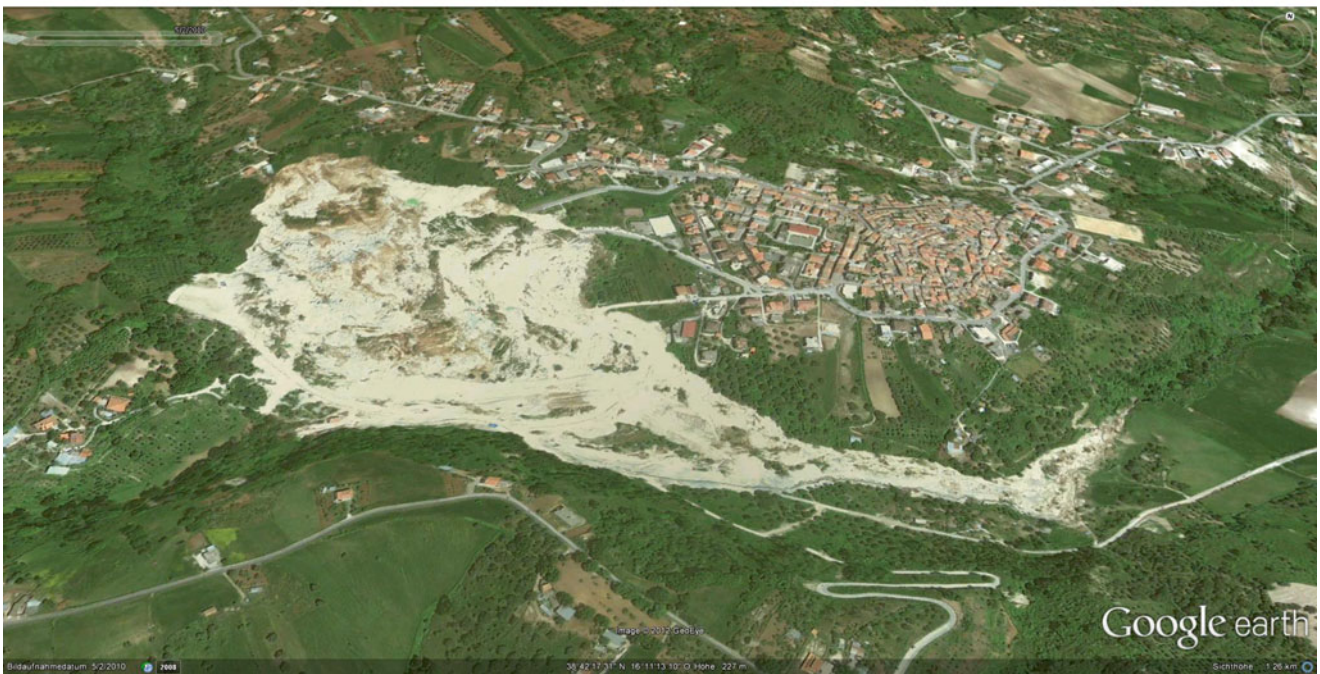
Fig. 8.7 (a, b) Sequence of images before and after the Maierato rock-slide on February 15th, 2010, in Calabria, southern Italy. The slide was induced by heavy rainfall during the days before the slide, which
