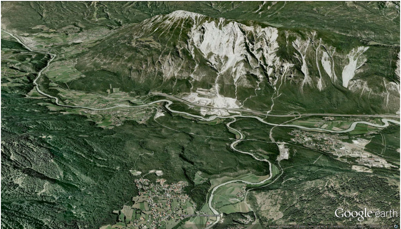
Fig. 8.6 The mass movement events (rockslides, sometimes also referred to as rock avalanches) at Tschirgant Mountain occurred along the Innthal fault system, related to internal rock deformation and fracturing. The Toma landscape of the debris is clearly visible (image center).
