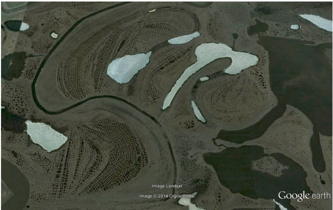
Fig. 13.15 With low temperatures ( -25 to -40 °C) in winter, the frozen ground shrinks repeatedly and cracks open up in networks, which will be filled by meltwater in the warmer times of the year. The water travels deeper and opens the cracks further in each thawing/freezing
