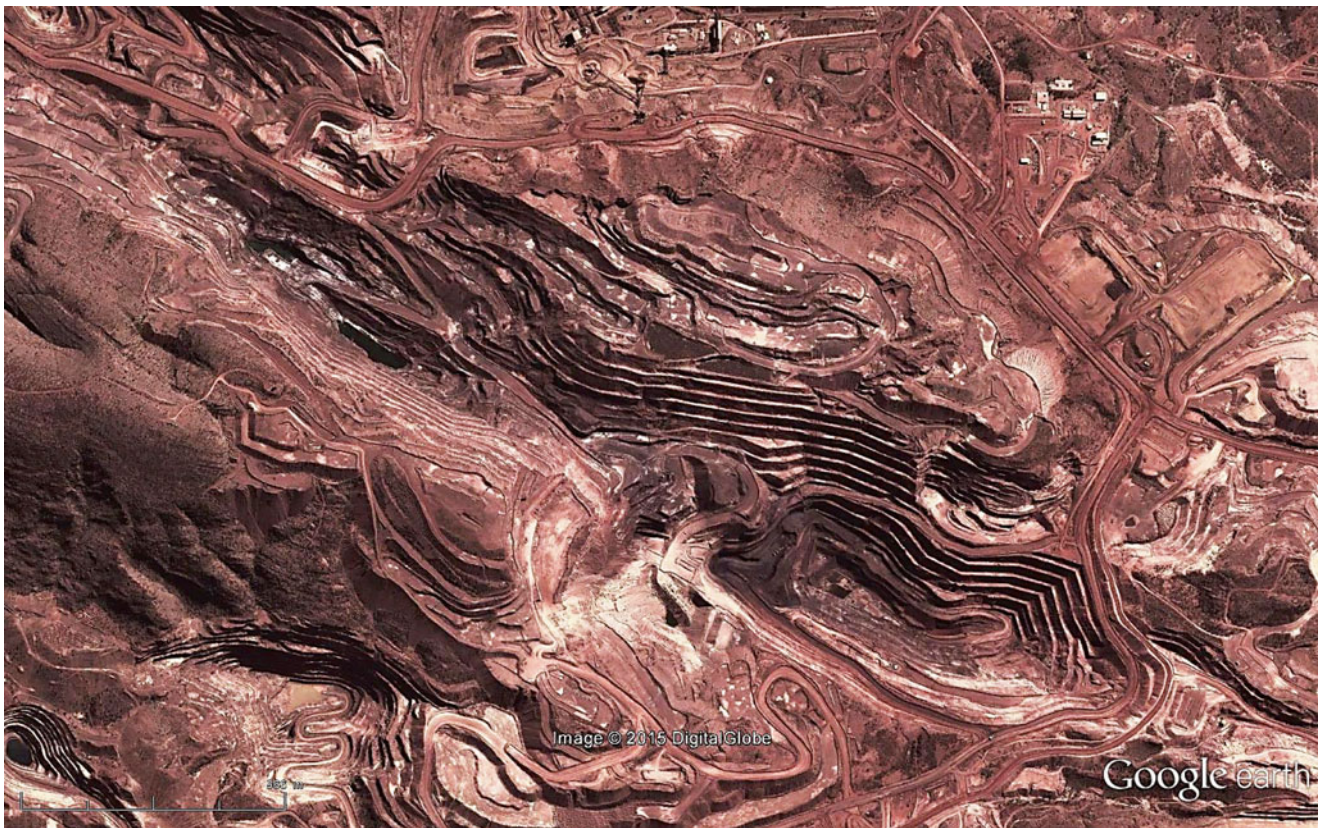
Fig. 14.8 Tom Price iron ore mine, Australia, at 22^{\circ}46'S and 117^{\circ}46'E . Scene is 10 km wide, showing greater than 40 km 2 of open mining up to 200 m deep; 28 million tons iron ore is moved per year (Image credit: ©Google earth 2012)
