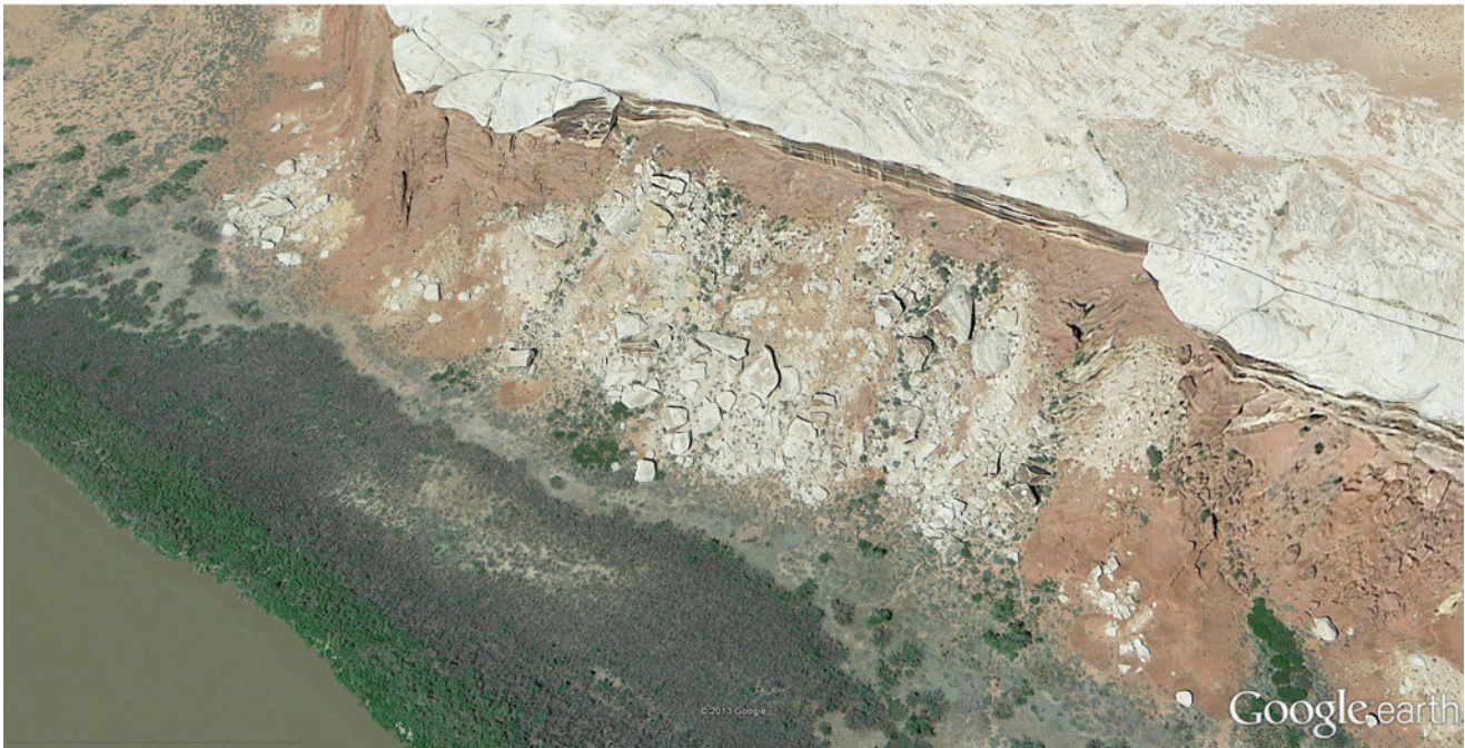
Fig. 8.1 (a) Rockfall of single large boulders along the “White Rim” of Canyonlands National Park in Utah, USA. Large parts of the softer underlying rock layers are covered by block- and boulder-sized rock debris. Their shape and size is predefined by the joint pattern in the overlying carbonate sandstone. Image shows a similar location as in
