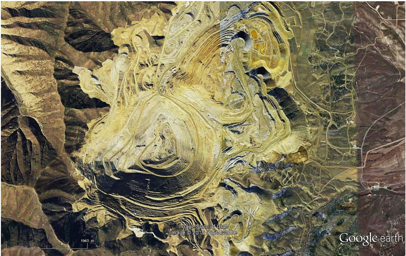
Fig. 14.9 Bingham Canyon open pit copper mine in Utah, USA, at 40^{\circ}32'N and 112^{\circ}09'W . Scene is about 15 km wide, showing the 8.5 km by 5.5 km open pit that is 600 m deep in the eastern end and 900 m deep
