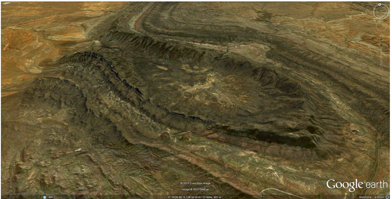
Fig. 4.13 The famous synclinal structure of Wilpena Pound, Flinders Ranges (South Australia) forms an almost closed basin. Mountain ranges surrounding the remnant valley have been eroded away during the last several million years. The higher walls of Wilpena Pound are
