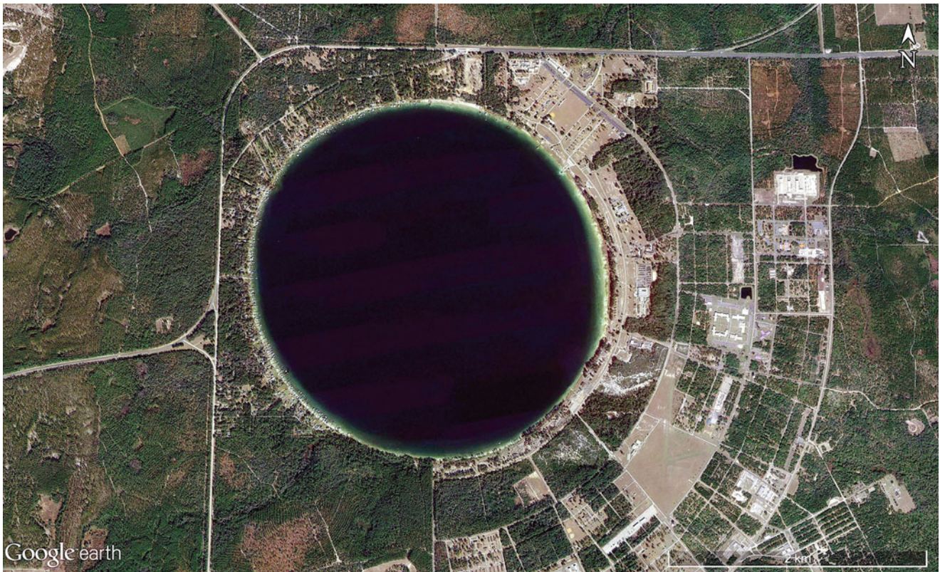
Fig. 2.69 Many Florida sinkholes, in particular those showing lakes, are almost perfectly round deep shafts connected to underground water levels with cave systems. This sinkhole at 29^{\circ}58'N and 82^{\circ}00'W has a diameter of 2.9 km (Image credit: ©Google earth 2013)
