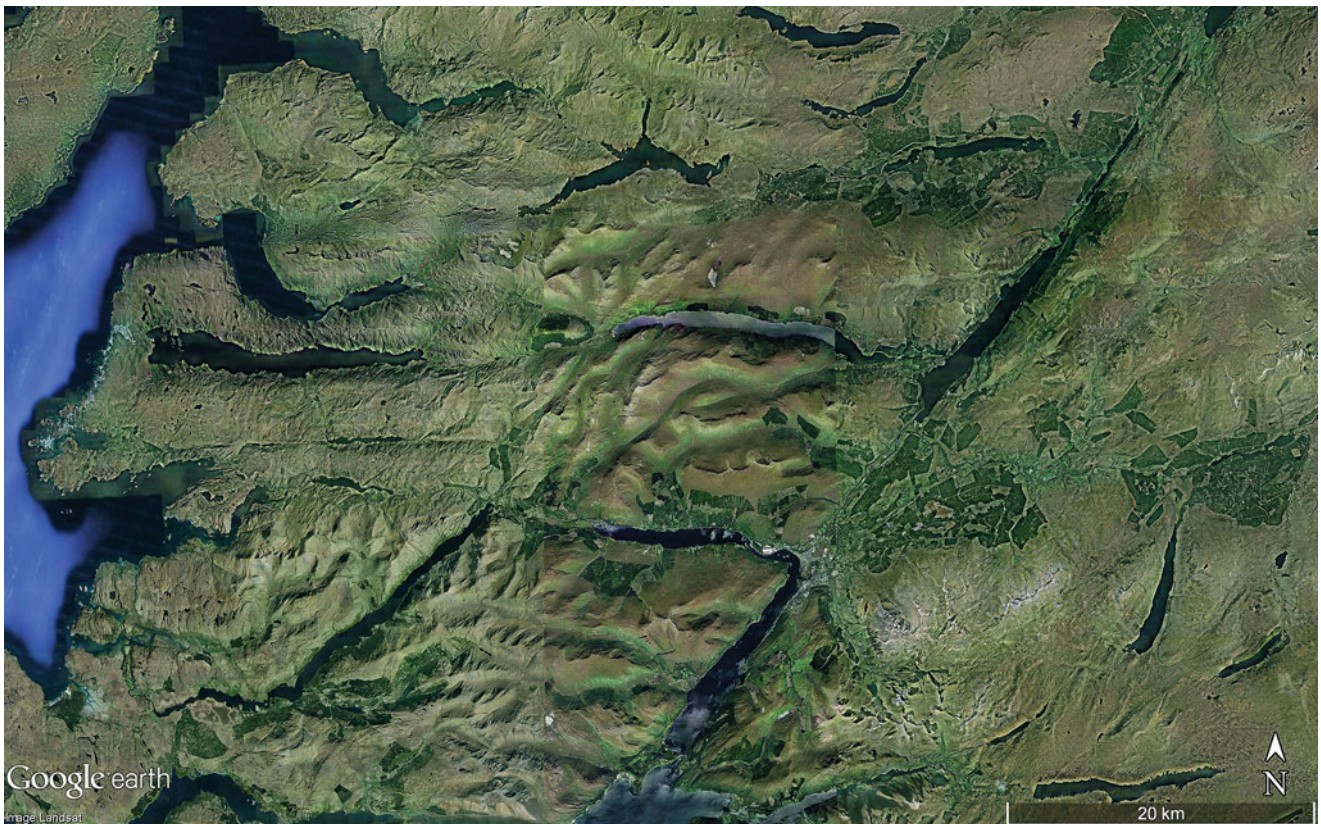
Fig. 2.14 Crossing of two main structural lines in northwest Scotland ( 56^{\circ}57'N , 5^{\circ}22'W ): W-E-structures are old and the younger SW-NE-lineament is the Caledonian Fault also known as the Great Glen Fault
