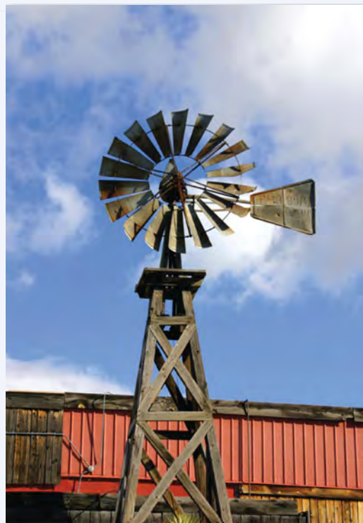
FIGURE 6-D Farm windmills such as the one on the left remain familiar sights in some areas. Mechanical energy from wind is commonly used to pump water. (Photo by Mehmet Dilsiz/Shutterstock) The wind turbines on the right are operating near Palm Springs, California. Although California is the state where significant wind-power development began, it has been surpassed by Texas and Iowa. (Photo by John Mead/Science Photo Library/Photo Researchers, Inc.)
