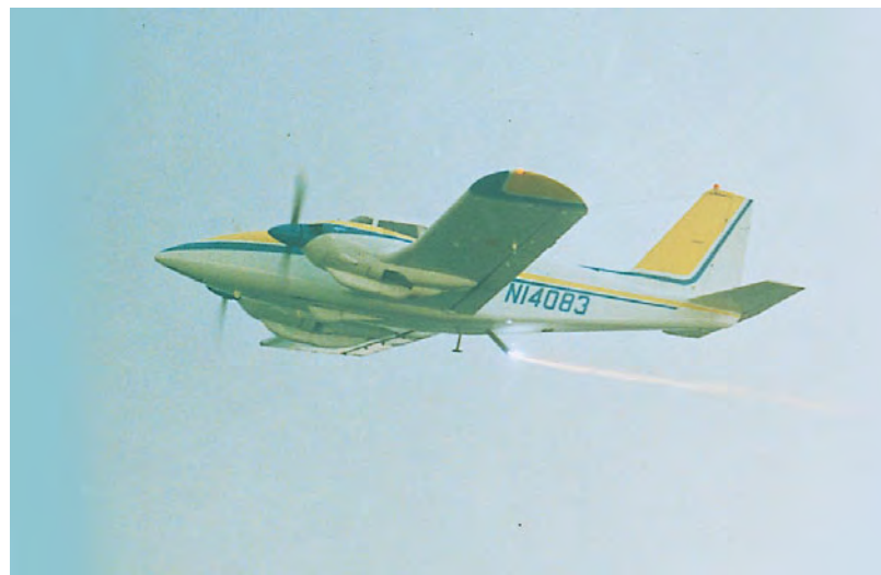
Figure 5-27 Cloud seeding using silver iodide flares is one way that freezing nuclei are supplied to clouds. (Courtesy of University Corporation for Atmospheric Research/National Science Foundation/National Center for Atmospheric Research)
