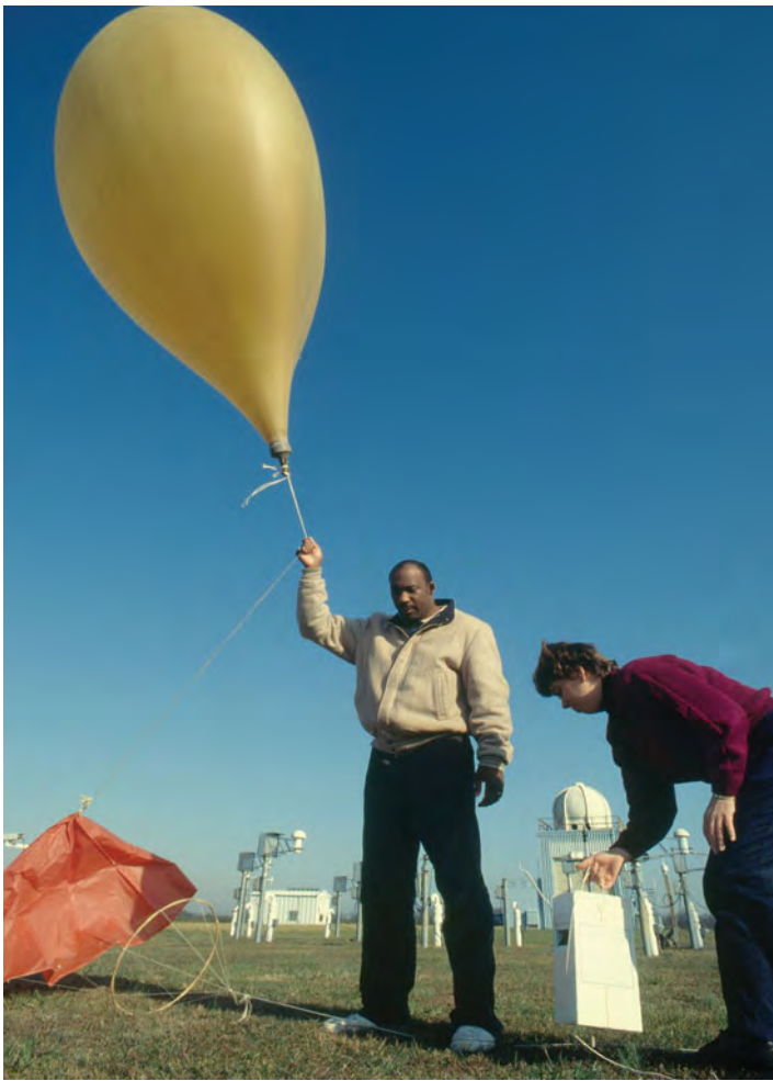
Figure 1-24 A lightweight instrument package, the radiosonde , is suspended below a 2-meter-wide weather balloon. As the radiosonde is carried aloft, sensors measure pressure, temperature, and relative humidity. A radio transmitter sends the measurements to a ground receiver. By tracking the radiosonde in flight, information on wind speed and direction aloft is also obtained. Observations where winds aloft are obtained are called “rawinsonde” observations. Worldwide, there are about 900 upper-air observation stations. Through international agreements, data are exchanged among countries. (Photo by Mark Burnett/Photo Researchers, Inc.)
