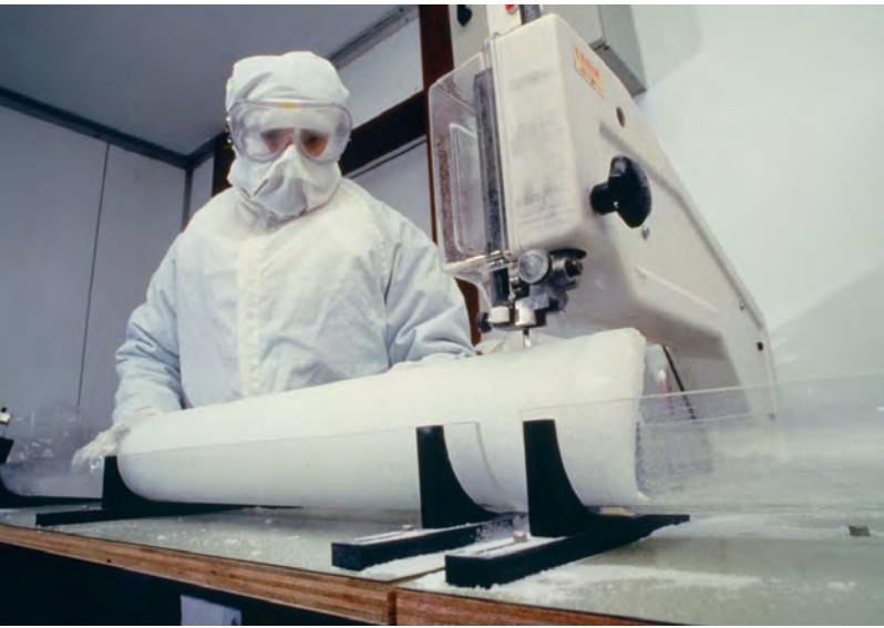
Figure 14-5 Scientist slicing an ice core sample from Antarctica for analysis. He is wearing protective clothing and a mask to minimize contamination of the sample. Chemical analysis of ice cores can provide important data about past climates. (Photo by British Antarctic Survey/Photo Researchers, Inc.)
