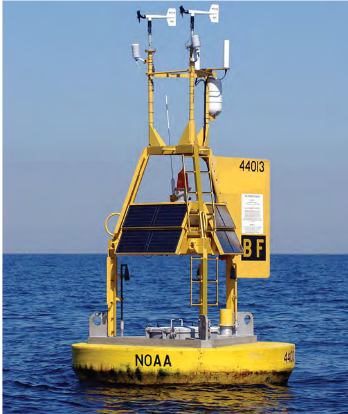
Figure 12-3 Data buoy used to record atmospheric conditions over a section of the global ocean. The data this buoy collects are transmitted via satellite to a land-based station. (Photo by Michael Dwyer/Alamy)
