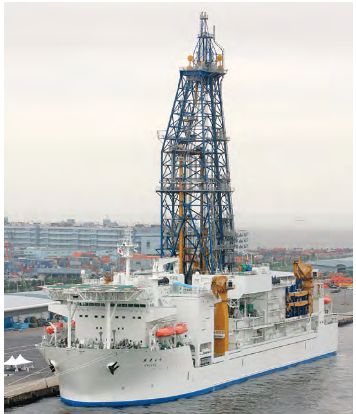
Figure 14-4 The Chikyu (meaning “Earth” in Japanese), the world’s most advanced scientific drilling vessel. It can drill as deep as 7000 meters (nearly 23,000 feet) below the seabed in water as deep as 2500 meters (8200 feet). It is part of the Integrated Ocean Drilling Program. (AP Photo/Itsuo Inouye)
