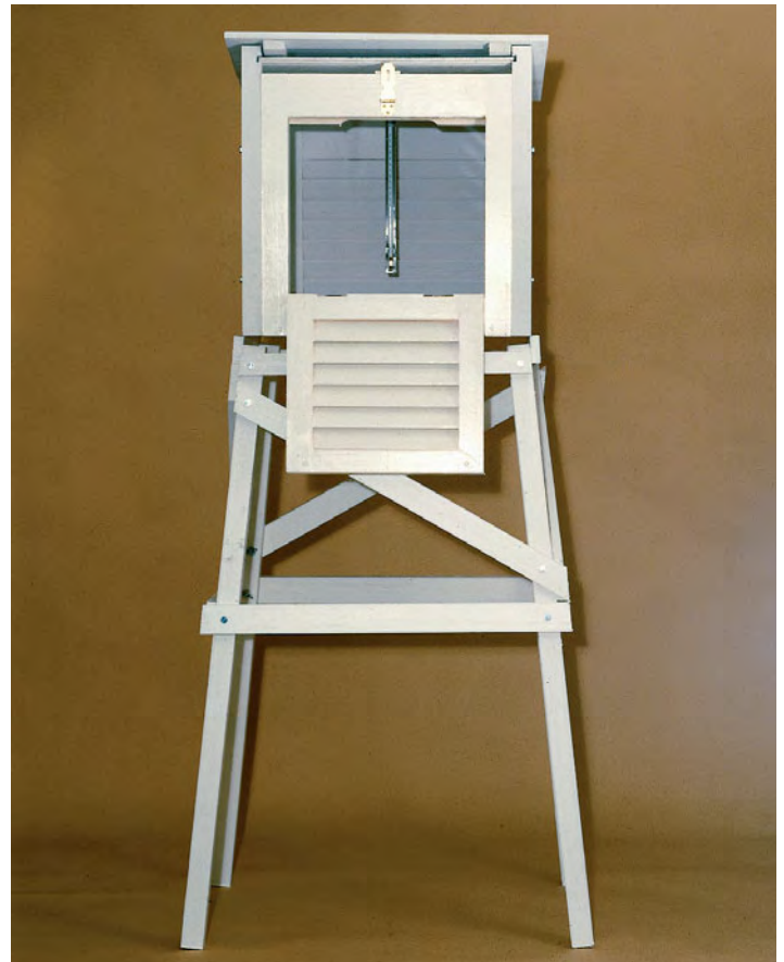
Figure 3–29 This traditional standard instrument shelter is white (for high albedo) and louvered (for ventilation). It protects instruments from direct sunlight and allows for the free flow of air. (Courtesy of Qualimetrics, Inc.)
