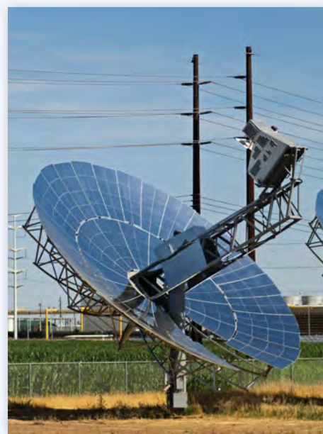
FIGURE 2-E This Stirling dish is located near Phoenix, Arizona. (Photo by Brian Green/Alamy)
