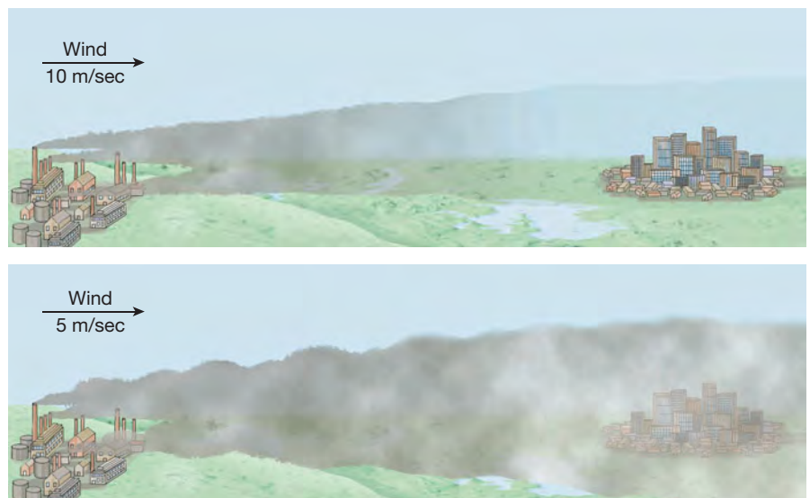
Figure 13-14 Effect of wind speed on the dilution of pollutants. The concentration of pollutants increases as wind speed decreases.
