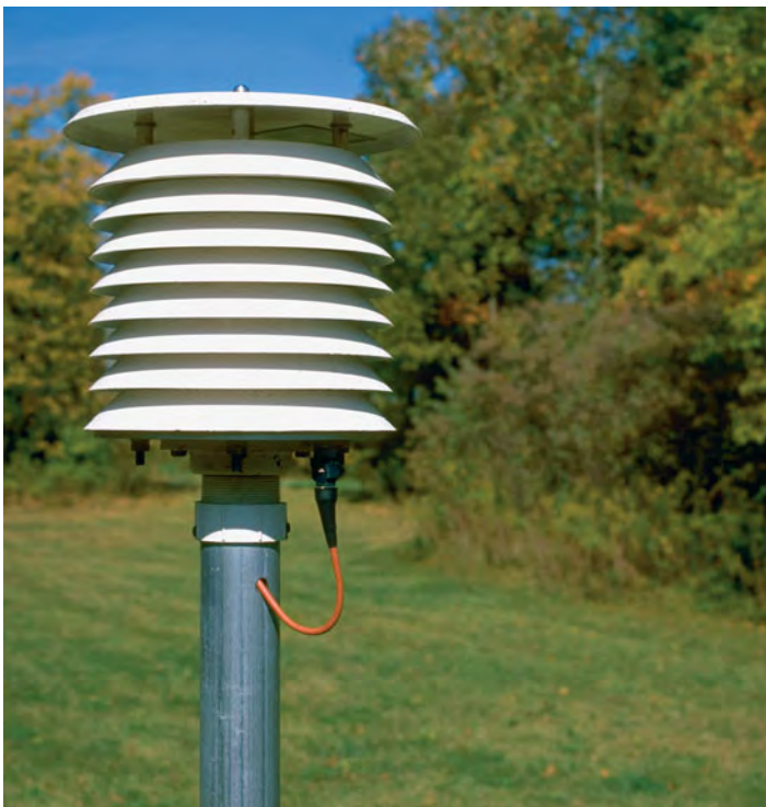
Figure 3–28 This modern shelter contains an electrical thermometer called a thermistor . (Photo by Bobbé Christopherson)
