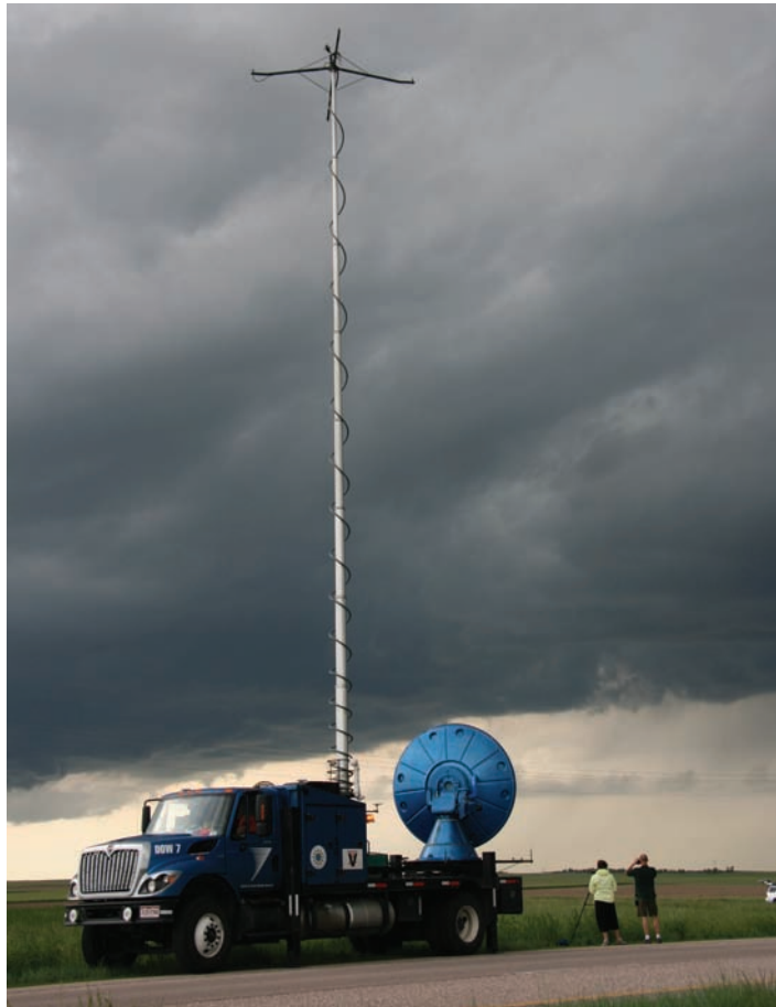
● FIGURE 15.27 A Doppler on Wheels mobile radar probes the thunderstorm that produced a tornado near Lagrange, Wyoming, on June 5, 2009. The unit was one of several involved with the VORTEX2 field study.
