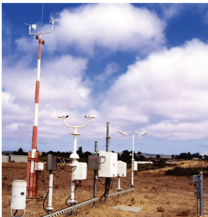
● FIGURE 3.35 The instruments that comprise the ASOS system. The max-min temperature shelter is the middle white box.
