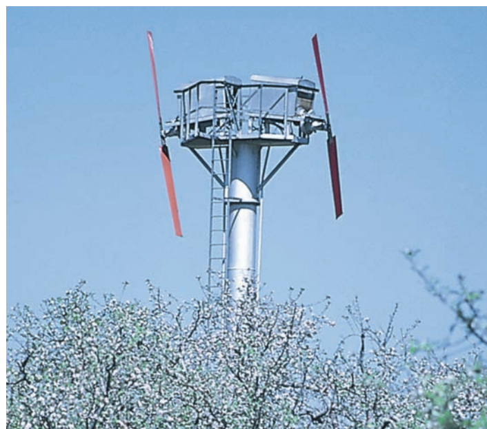
● FIGURE 3.20 Wind machines mix cooler surface air with warmer air above.
