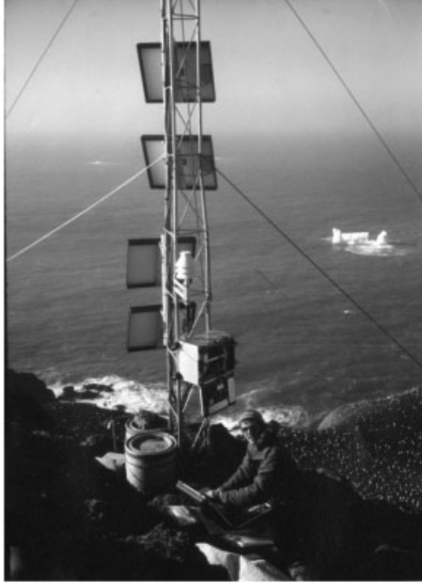
Figure 23 Interagency automatic remote collector (ARC) using satellite communications on Macaroni Ridge in Antarctica. Weather data are used in penguin breeding studies. Hundreds of penguins in lower right background. See ftp site for color image.
