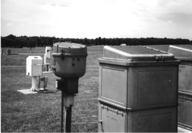
Figure 16 Fixed-beam ceilometer (cylindrical shaped) and rotating-beam ceilometer detector on right. See ftp site for color image.
