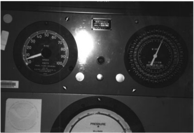
Figure 12 Wind speed and wind direction indicators. See ftp site for color image.
