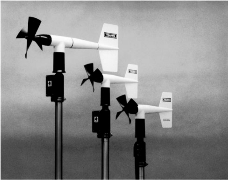
Figure 5 (Top) Model 05103 Wind Monitor (standard model, shown for relative size). (Middle) Model 04101 Wind Monitor-JR (junior model), November, 1993. (Bottom) Model 04106 Wind Monitor-JR/MA (junior marine model), October, 1994. See ftp site for color image.
