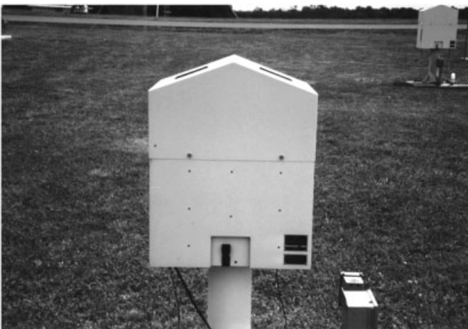
Figure 18 Laser beam ceilometer showing transmitter and receptor windows. See ftp site for color image.
