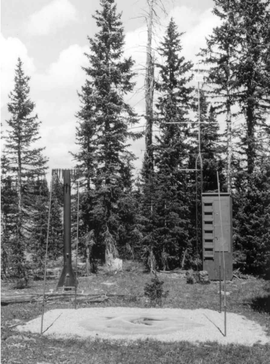
Figure 7 U.S. Department of Agriculture Natural Resources Conservation Service SNOTEL (Snow Telemetry) site in the western United States including snow pillow (in foreground), a shielded standpipe precipitation storage gage (left background), and radio telemetry equipment (from Doesken and Judson, 1997).
