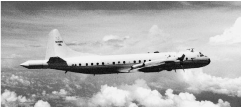
Figure 19 ELDORA airborne radar can be deployed quickly to almost any point in the world, even over oceans. It has a sophisticated radar in the protuberance extending beyond the normal tail. Similar systems are used operationally to intercept hurricanes. (Courtesy NCAR/ATD.) See ftp site for color image.
