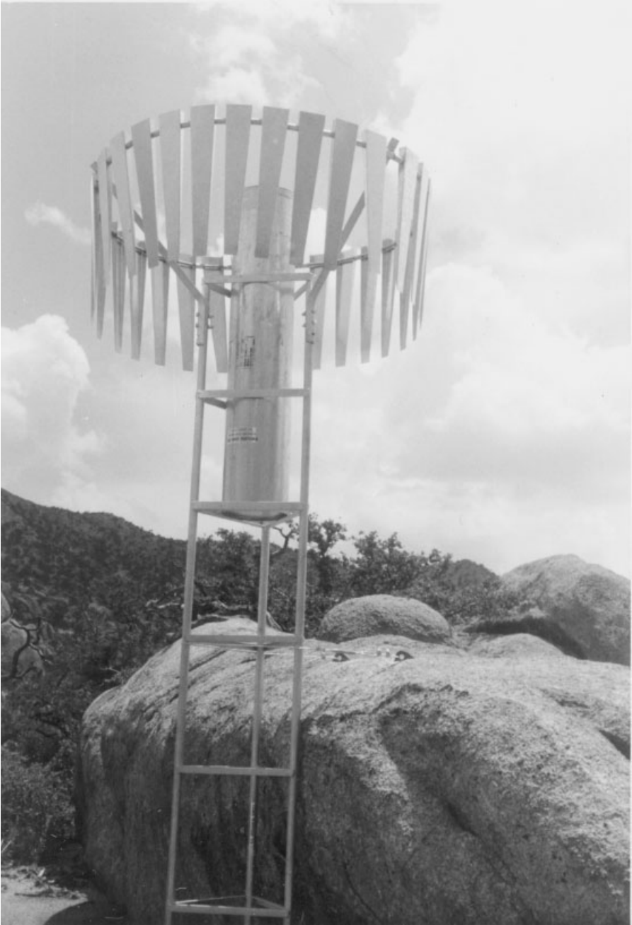
Figure 4 Alter wind shield on a tower-mounted precipitation gage (from Doesken and Judson, 1997).
