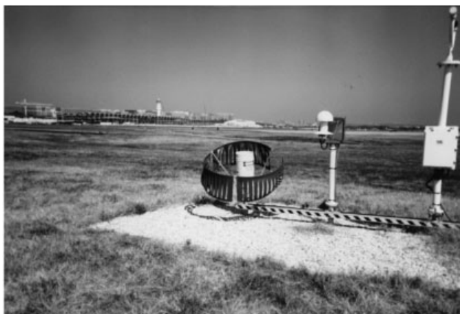
Figure 9 Sensors located too close to a jet takeoff area. Windscreen around the rain gauge is damaged from jet blast. Blast also causes temperature to rise and wind gusts to increase. See ftp site for color image.
