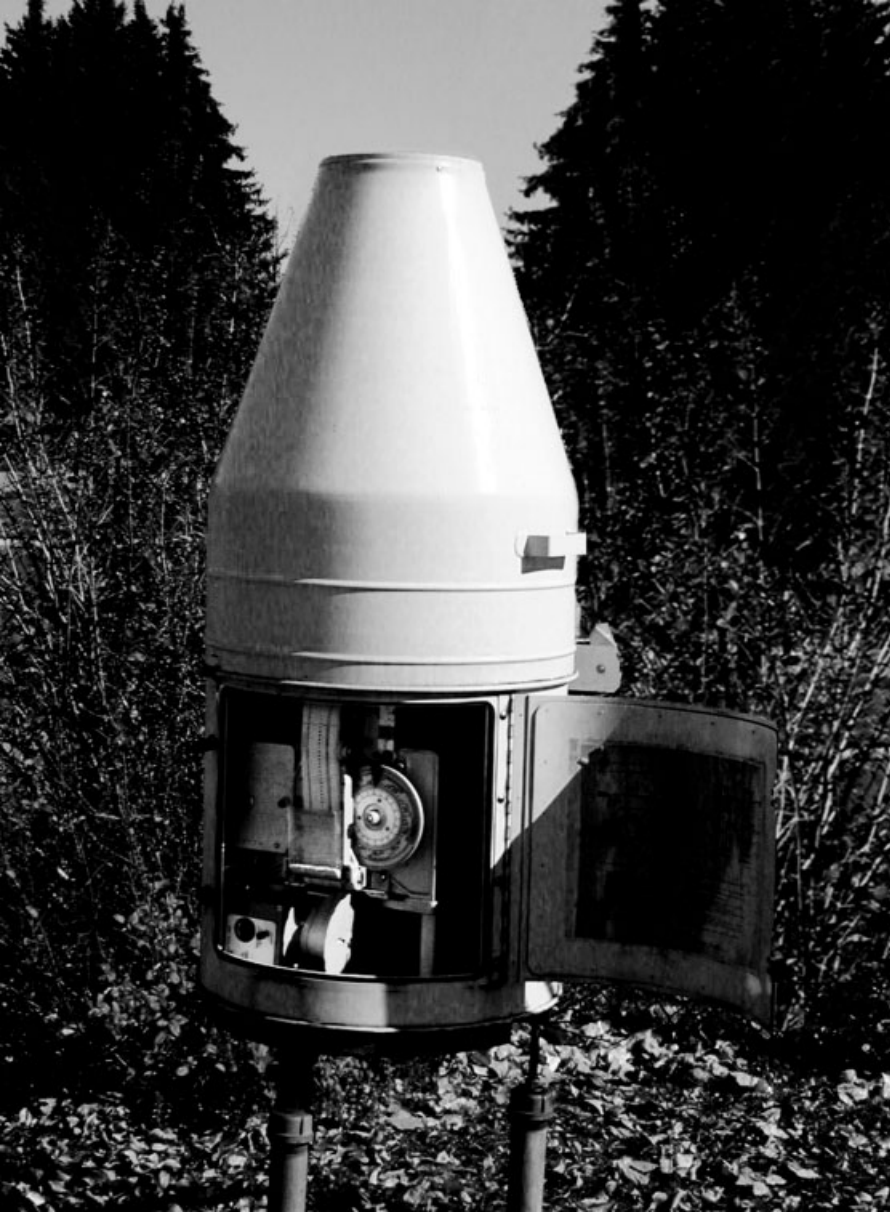
Figure 2 National Weather Service Fischer–Porter recording rain gage. Close to 3000 of these gages are in use in the United States for recording hourly and 15-min precipitation totals in increments of 0.10 in. (photo by Clara Chaffin).
