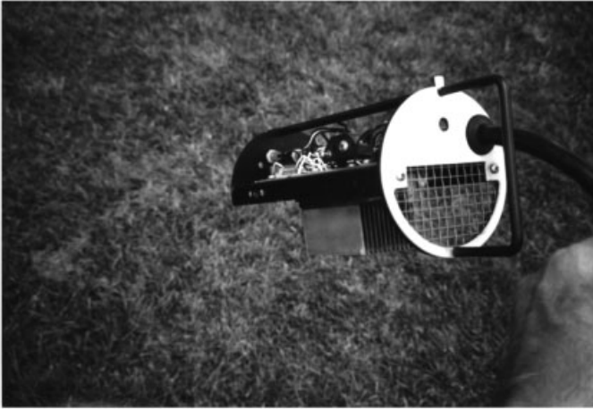
Figure 5 Hygrothermometer interior showing intake air screen. Finned object on bottom is Peltier device. See ftp site for color image.
