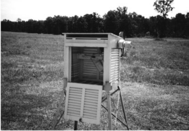
Figure 2 Cotton Region temperature shelter with door open. See ftp site for color image.
