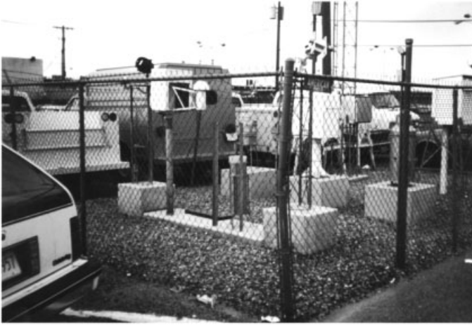
Figure 25 Sensors poorly exposed in a parking lot. See ftp site for color image.
