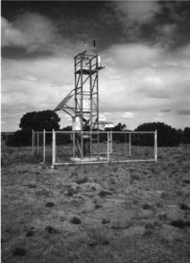
Figure 21 Early remote automated meteorological observing system (RAMOS), late 1960s. See ftp site for color image.
