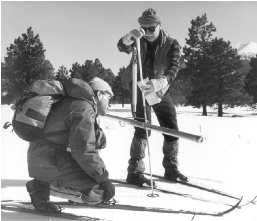
Figure 6 Federal snow sampler consists of a cutter, tubes, and scales for measuring snow water equivalent in moderate and deep snowpacks (from Doesken and Judson, 1997).
