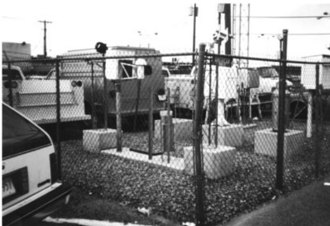
Figure 8 Sensors poorly exposed in a parking lot. See ftp site for color image.
