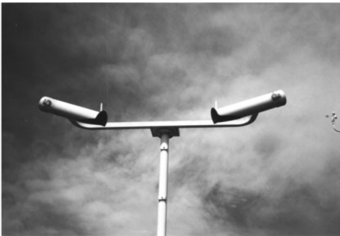
Figure 20 Forward scatter visibility sensor showing projector and receiver. See ftp site for color image.
