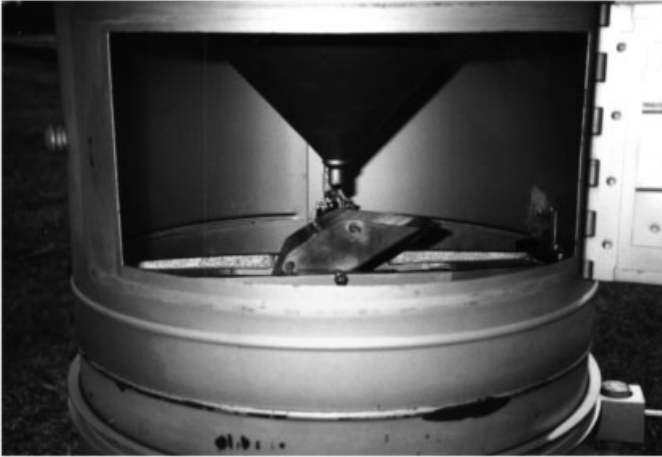
Figure 8 Tipping bucket mechanism. See ftp site for color image.
