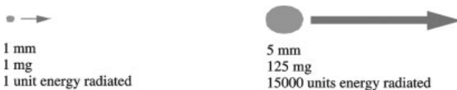
Figure 5 Relative diameter, mass, and scattered energy from small and large drops. Large drops scatter much more energy than small drops. See ftp site for color image.
