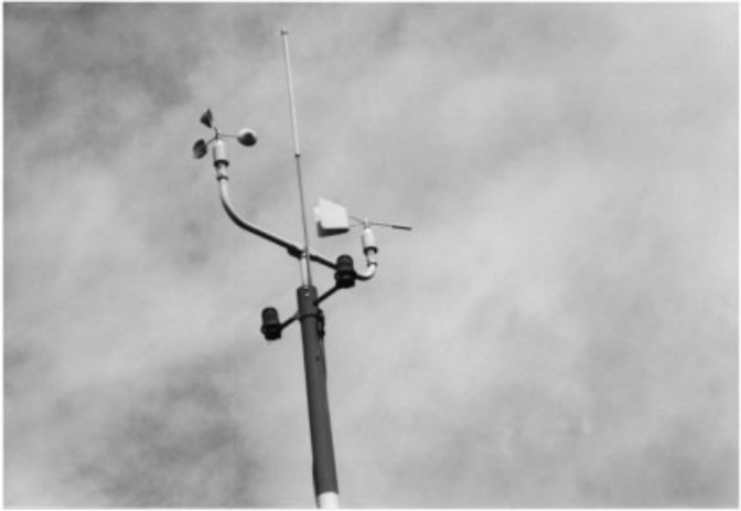
Figure 11 Rotating cup anemometer and wind direction sensor atop 10-m tower. See ftp site for color image.
