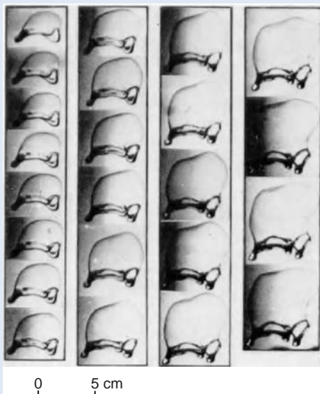
Fig. 6.26 Sequence of high-speed photographs (starting at upper left and moving down and to the right) showing how a large drop in free fall forms a parachute-like shape with a toroidal ring of water around its lower rim. The toroidal ring becomes distorted and develops cusps separated by threads of water. The cusps eventually break away to form large drops, and the thin film of water that forms the upper part of the parachute bursts to produce a spray of small droplets. Time interval between photographs = 1 ms. [Photograph courtesy of B. J. Mason.]
