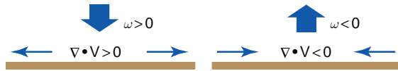
Fig. 7.18 Algebraic signs of \omega in the midtroposphere associated with convergence and divergence in the lower troposphere.
