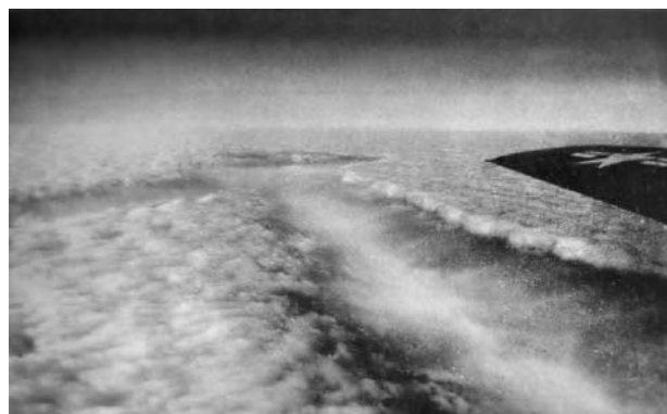
Fig. 6.47 A \gamma -shaped path cut in a layer of supercooled cloud by seeding with dry ice. [Photograph courtesy of General Electric Company, Schenectady, New York.]
