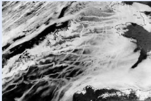
Fig. 6.9 Ship tracks (white lines) in marine stratus clouds over the Atlantic Ocean as viewed from the NASA Aqua satellite on January 27, 2003. Brittany and the southwest coast of England can be seen on the upper right side of the image.
