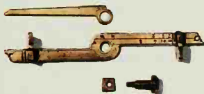
Rule (on front of instrument, over the rete), sighting arm (on the back), and pivot pin.
