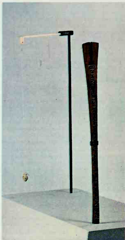
The merkhet, a device consisting of sighting rod and two plumb-lines, used in ancient Egypt for observing the transit of stars.
