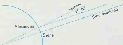
Figure 3.14 When noon Sun was directly overhead at Syene it made an angle of 7^{\circ}12' with the vertical at Alexandria. If both were on the same meridian, the distance between them was just one-fiftieth of Earth's circumference.
