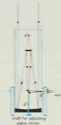
Above: Part of Nasmyth's 20-inch Cassegrain-Newtonian telescope, showing position of eye-piece in relation to mounting. Below: Nasmyth using the instrument, which could be pointed to any part of the heavens without the observer's having to move.
