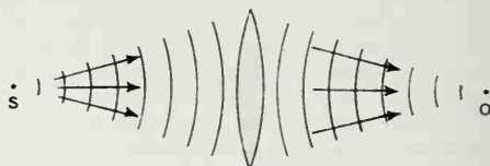
Figure 7.15 It can also explain how such a lens brings light from S to a focus at O.
