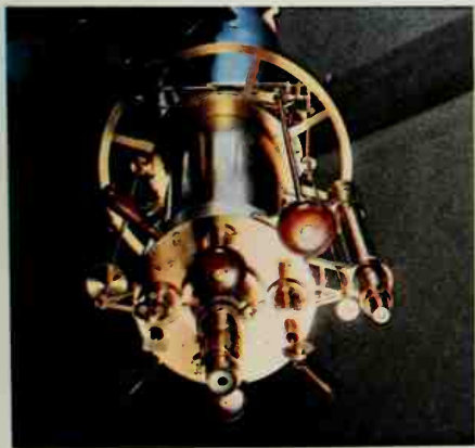
The instrument first used to measure star distances was the heliometer. On the left is a general view of the heliometer installed at the Oxford Observatory in 1848. To the right are close-ups of the eyepiece and the split objective.
