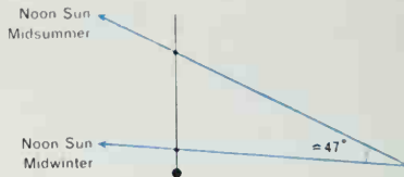
Figure 2.2 Fixing angle between observer, Sun's highest noon altitude and Sun's lowest noon altitude.
