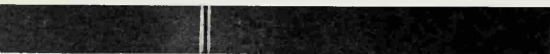
Part of spectrum produced by hot sodium vapor. The two strong lines (yellow) are the so-called D lines.
