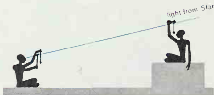
The merkhet, a device consisting of sighting rod and two plumb-lines, used in ancient Egypt for observing the transit of stars.
