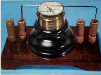
Ørsted first showed that while any charge produces an electric field only a moving charge will produce a magnetic field. Above is a model of the apparatus he used to show the effect that a direct current has on a compass needle pivoted below the wire which carries it.
