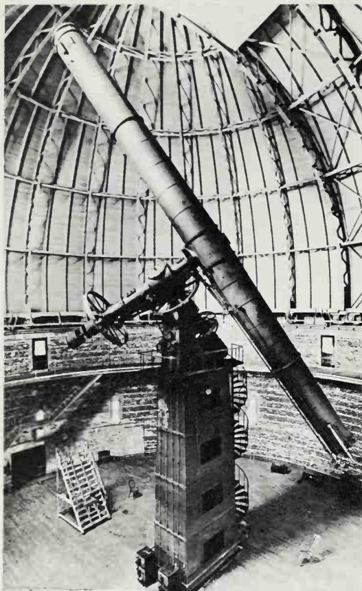
Not until near the end of last century was a telescope equipped with a lens of 3-foot diameter. Today the world's largest refractor is the 40-inch instrument at Yerkes, Williams Bay, shown above.
