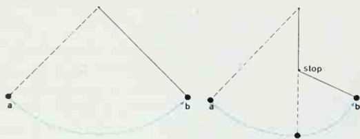
Galileo found that if the speed of a pendulum bob at the bottom of its swing remains unchanged, the height to which the bob rises is not affected by changing the length of the string. This suggested that the behavior of the bob does not depend on the existence of the string.
