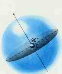
Figure 1.7 As a step to defining positions on the celestial sphere we can specify the equator, then draw through its center (C) a line perpendicular to it. This line is the polar axis.
