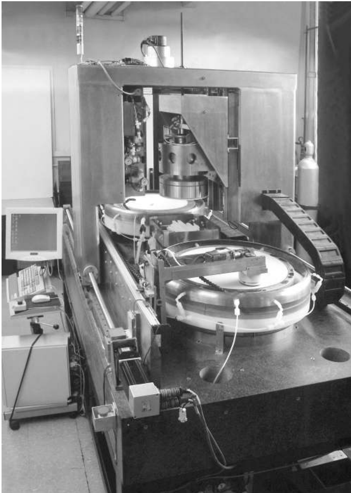
Figure 6-2: Photograph of the fabricated MIT CMP Platform
