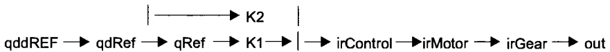
Fig. 4.42. Composition diagram of one axis of the industrial robot, shown in Fig. 4.42
