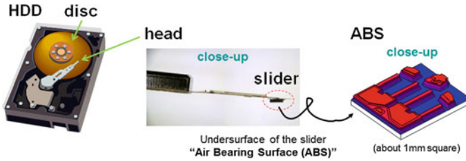
Fig. 2 Slider of HDD and its air bearing surface (ABS)
