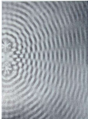
Figure 10.18: The waves emitted by two synchronized sources form an interference pattern. Observe the stripes of destructive interference where the waves meet “out of sync” (peak to troughs) and cancel each other out.
