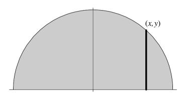
If the vertical rectangle shown is rotated about the x axis, a disk of radius y and thickness dx is generated. The volume of a typical disk is  $\pi y^2 dx$  and the total volume of the solid of revolution is
