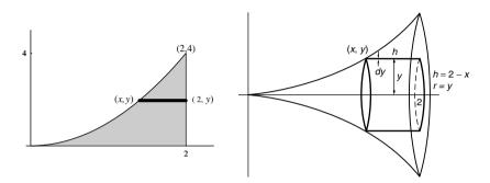
If (x, y) represents an arbitrary point on the graph  $y = x^2$ , the length of the generated shell is h = 2 - x, the radius r = y, and the thickness of the shell is dy. The volume of a typical shell is  $2\pi y(2-x) dy$  and the total volume of the solid is obtained by integration. Since the volume of the shell involves dy, integration will be with respect to y. Since  $y = x^2$ , y = 0 when x = 0 and y = 4 when x = 2. Therefore,
