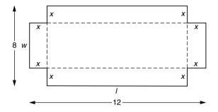
Since the length and width of the box will be the corresponding dimensions of the sheet metal diminished by 2x, l = 12 - 2x, w = 8 - 2x, and the height of the box will be just x itself. By substitution.
