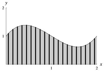
The diagram shows the function  $y = x^3 - 3x^2 + 2x + 1$  drawn with about 20 "imaginary" vertical rectangles of height y and thickness dx. If we imagine an *infinite number* of such rectangles extending from x = 0 to x = 2, each *infinitesimally thin*, the rectangles will "color in" the required area. Since integra-
