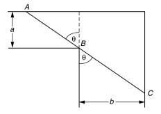
Let  $\boldsymbol{\theta}$  be the angle between the pipe and the vertical as shown in the diagram.
