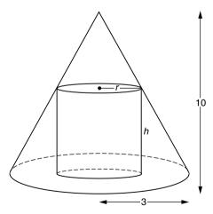
The volume of a cylinder is  $V = \pi r^2 h$ . To obtain a relationship between r and h, we examine the figure from a two-dimensional perspective.
