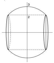
The sphere is generated by rotating the upper half of the circle  $x^2 + y^2 = 9$  about the x axis. We solve this problem using the shell method, using shells of radius y and length 2x.
