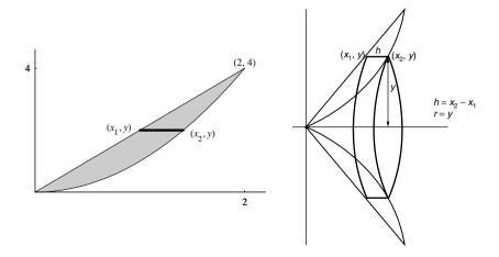
The length of each shell  $h = x_2 - x_1$  and the radius r = y. The thickness of each shell is dy. Therefore, the volume of a typical shell is  $2\pi(x_2 - x_1)y \, dy$  and the total volume is
