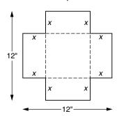
The volume of the box is V = lwh where l = 12 - 2x, w = 12 - 2x, and h = x. Substituting,
