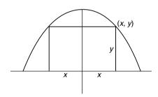
The height of the rectangle is y and the width is 2x. The rectangle's area is A = 2xy.
