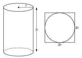
The material used in the construction of the can consists of three pieces. The area of the body of the can is  $2\pi rh$  and the material
