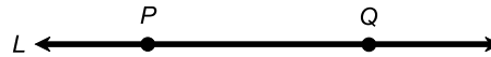
Fig. 1-1. Two point principle. For two specific points P and Q , line L is unique.
