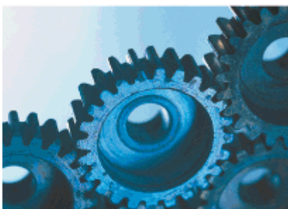
The teeth in the gears shown extend from circles that are externally tangent.
