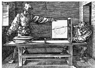
Figure 1 An artist using Dürer's perspective machine. © Copyright: The Trustees of the British Museum.
