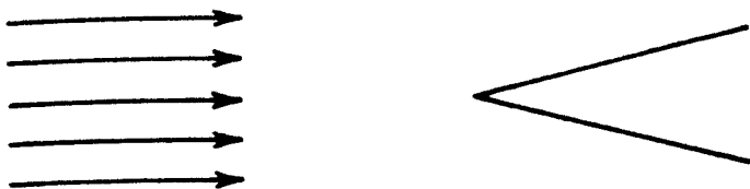
Fig. 6.2. Air current blowing against the edge of a wedge, viewed in cross-section
