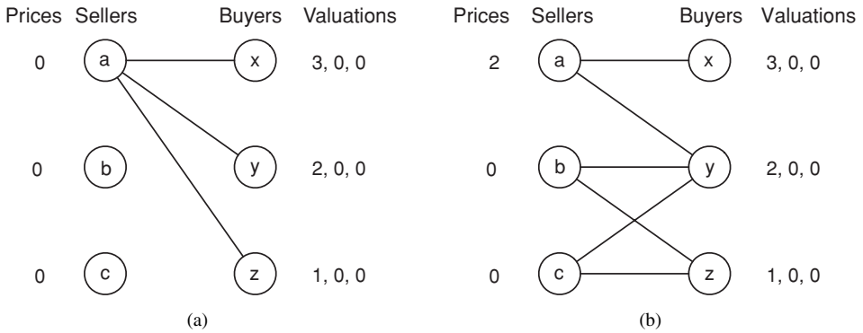
Figure 10.7. A single-item auction can be represented by the bipartite graph model: the item is represented by one seller node, and then there are additional seller nodes for which all buyers have 0 valuation. (a) The start of the bipartite graph auction. (b) The end of the bipartite graph auction, when buyer x gets the item at the valuation of buyer y .
