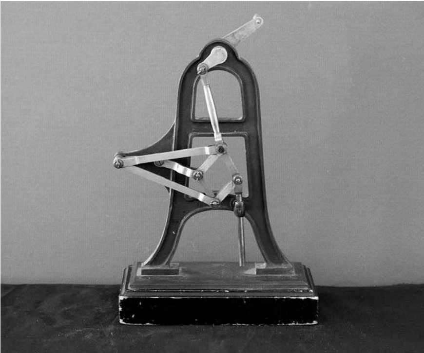
Figure 17a: The Peaucellier linkage (photographed by Francis C. Moon)
