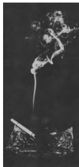
Figure 13 Transition from laminar to turbulent flow in cigarette smoke. Reprinted with permission from Physics Today , April 1983, p. 43, Copyright © 1983 American Institute of Physics.
