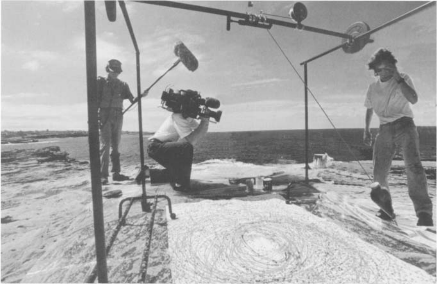
FIGURE 3 A photograph of the guided pendulum apparatus (referred to as the “Pollockiser”) used to generate drip paintings. The photograph was taken during filming for the Australian Broadcasting Corporation’s television program Quantum in March 1998.
