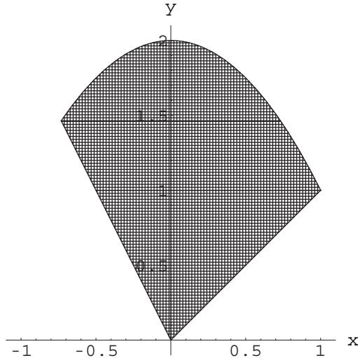
Note that the intersection point of  $y = -2x$  and  $y = 2 - x^2$  is  $(1 - \sqrt{3}, -2 + 2\sqrt{3})$ . We use the  $y$ -axis to divide the region into two type 1 subregions. Then
