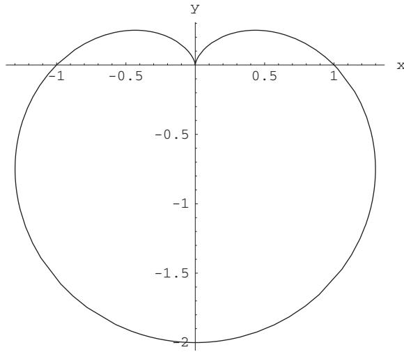
We first calculate  $M = \int_0^{2\pi} \int_0^{1-\sin \theta} r dr d\theta = \frac{3\pi}{2}$  and  $M_x = \iint_D y dA = \int_0^{2\pi} \int_0^{1-\sin \theta} r^2 \sin \theta dr d\theta = \frac{-5\pi}{4}$ , so  $\bar{y} = \frac{-5\pi/4}{3\pi/2} = -5/6$ .
