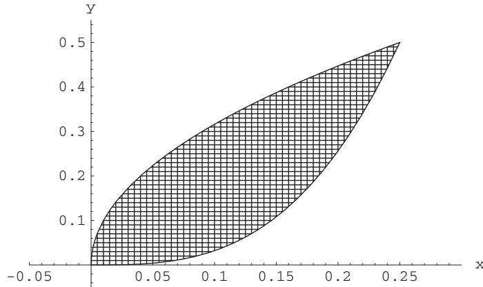
$$\begin{aligned} \int_0^{1/4} \int_{32x^3}^{\sqrt{x}} 3xy dy dx &= \int_0^{1/4} \left( \frac{3xy^2}{2} \right) \Big|_{32x^3}^{\sqrt{x}} dx = \int_0^{1/4} \left( \frac{3}{2}x^2 - 1536x^7 \right) dx \\ &= \left( \frac{3}{2}x^2 - 192x^8 \right) \Big|_0^{1/4} = \frac{1}{128} - \frac{3}{1024} = \frac{5}{1024}. \end{aligned}$$
