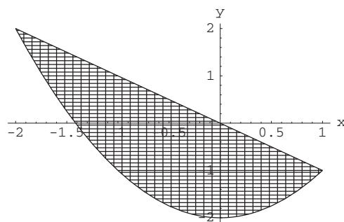
To reverse the order of integration we must divide  $D$  into two regions by the line  $y = -1$ . Then the original integral is equivalent to the sum
