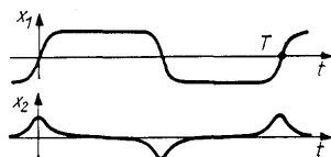
Fig. 108. The angle of deviation of the pendulum and its rate of change for amplitude near \pi
