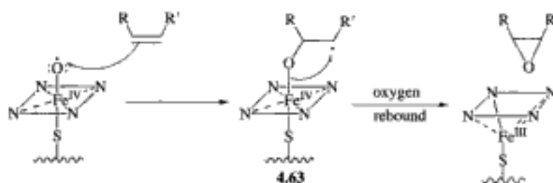
Scheme 4.37 ▶ Mechanism for heme-dependent epoxidation reactions
