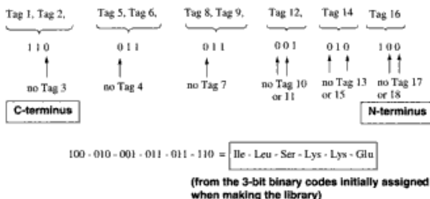
Figure 2.6 ► An example of encoding the structure of a peptide bound to a polymer bead by the Still methodology
