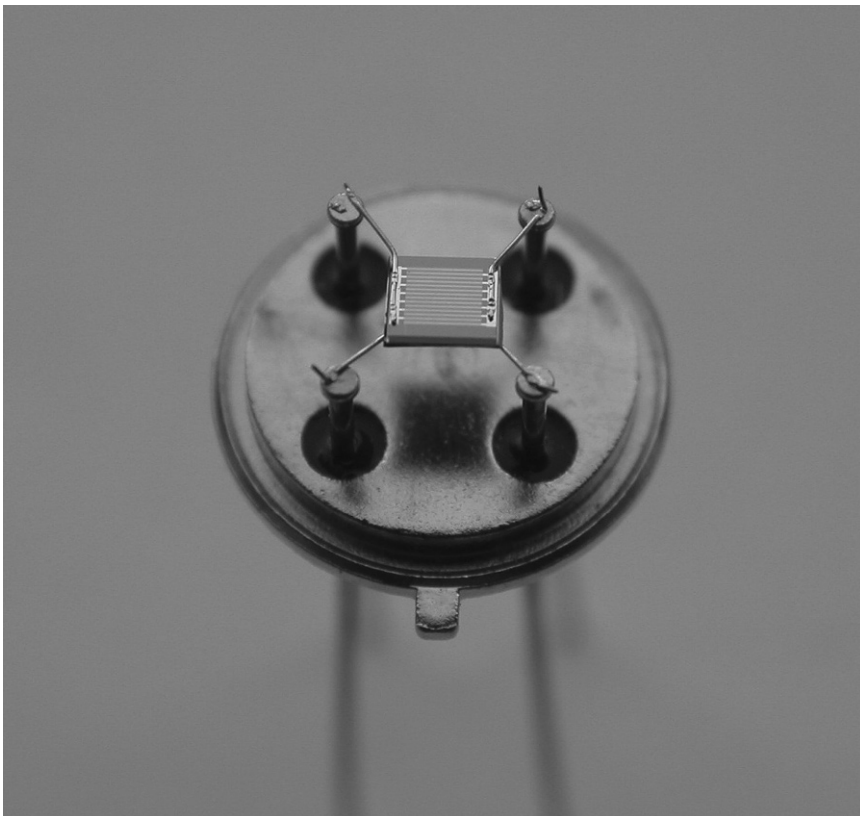
5.1 Packaged thin film gas sensor on silicon substrate (die 2 \times 2 \text{ mm}^2 ). (Source: Courtesy of L. Francioso.)
