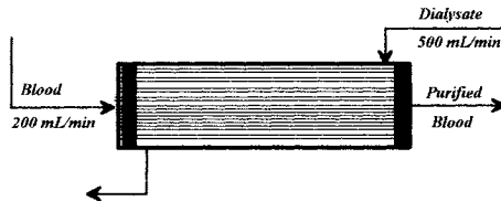
Figure 2.5-1. Schematic of haemodialysis unit. Blood is passed along fibre lumen, and solutes are exchanged with dialfiltrate
