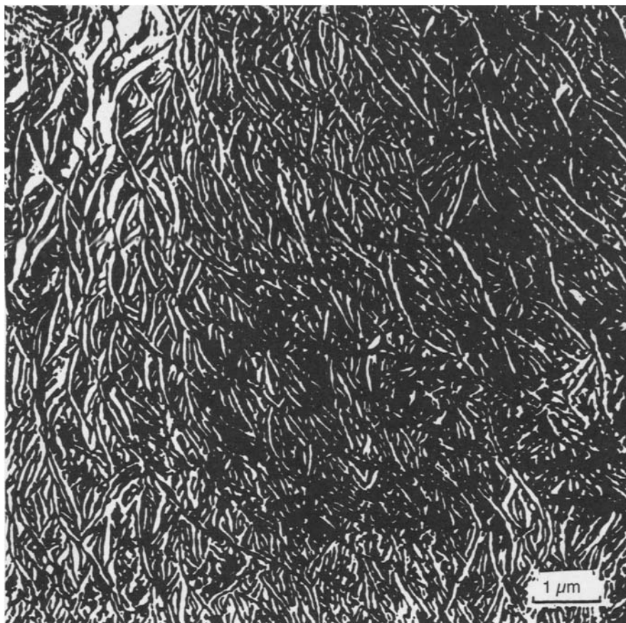
Fig. 22.2 Lamellar structure of poly(ethylene).
