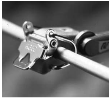
Fig. 6.7. Pressure sensor for Diesel injection lines. Such pressure sensors have a multimillion pieces per year market (taken from [4])
