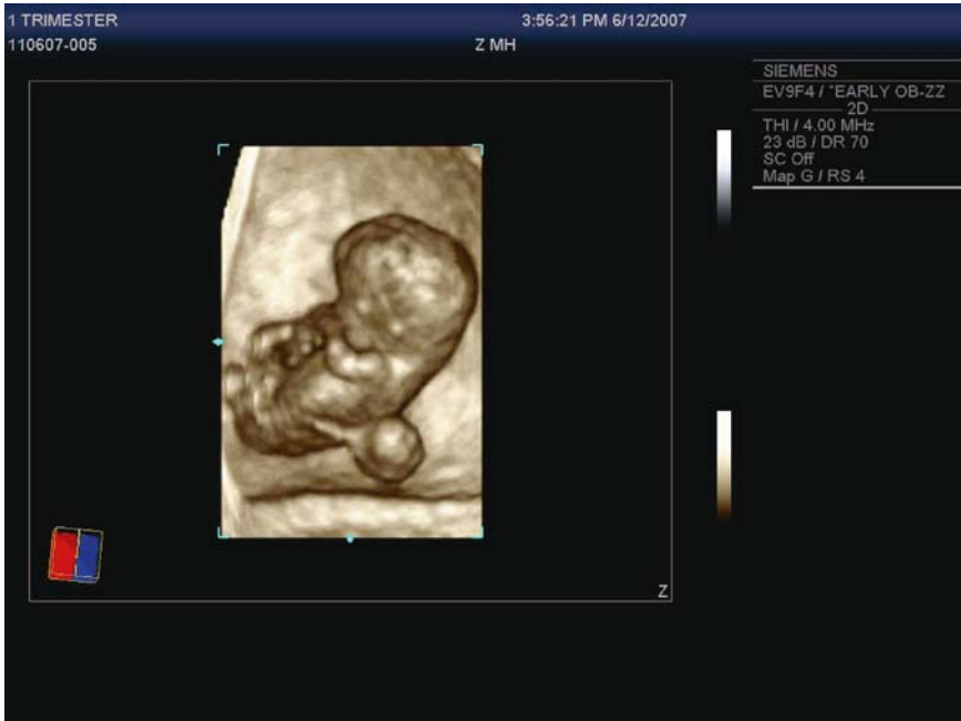
Fig. 8.16. Ultrasonic image of a foetus (tenth week pregnancy) taken with a mechanically moved 1D linear multilayer antenna
