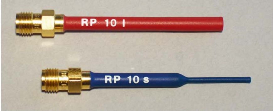
Fig. 6.6. Commercially available PVDF hydrophones (taken from [3])
