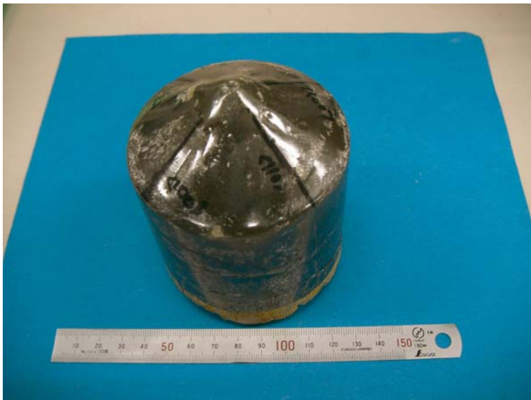
Fig. 9.12. Large size, 80 mm in diameter PMN-PIN-PT single crystal produced by the Bridgman process (Courtesy of JFE Minerals Co. of Japan, see [20])
