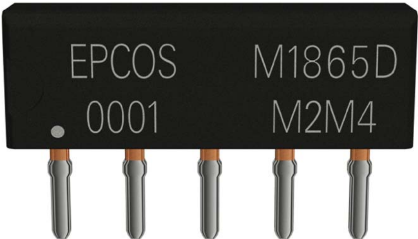
Fig. 14.19. Typical SAW TV-IF filters in five-pin single in line lead frame packages
