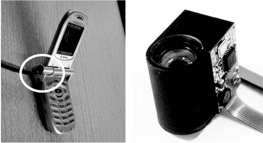
Fig. 11.20. Camera auto zooming/focusing mechanism with two metal tube USM's in a Samsung cellular phone
