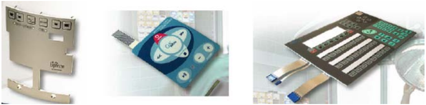
Fig. 6.12. Flexible keypads of different geometry, realized with piezoelectric laquer technology (taken from [6])
