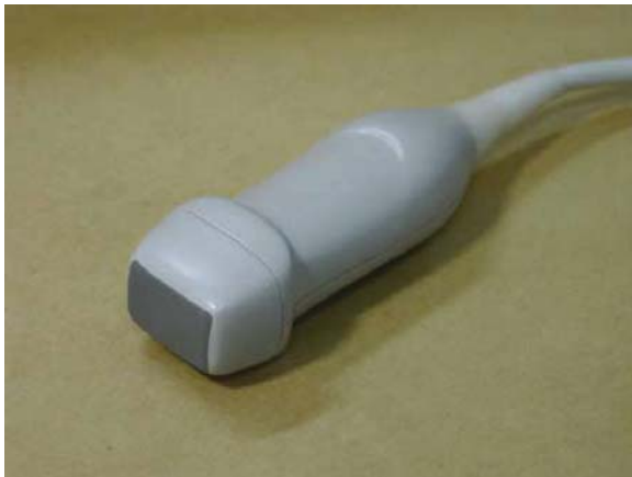
Fig. 9.15. The first commercialized 2.6 MHz PMNT single crystal medical probe (Courtesy of Humanscan Co. of Korea, see [25])
