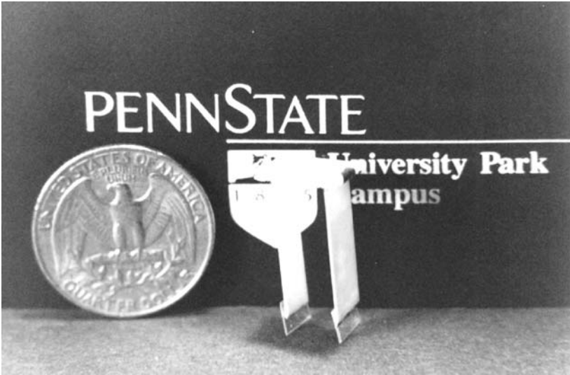
Fig. 11.5. A photo-driven micro walking device, designed to begin moving by light illumination. It is simple in structure, having neither lead wires nor electric circuitry
