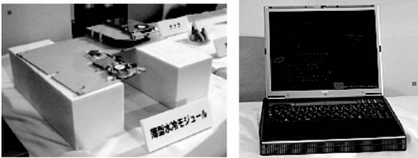
Fig. 11.15. A piezoelectric pump water cooling module (left) for a fuel cell in a laptop computer (Courtesy by NEC)
