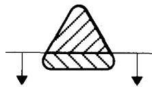
Grind a face from one side of the file to obtain two sharp edges
