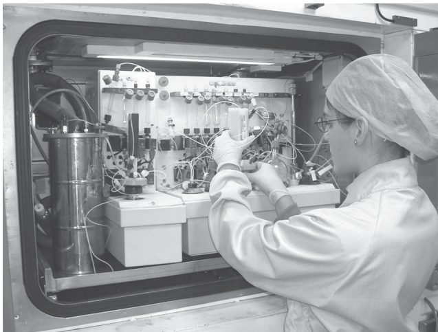
FIGURE 7 Automated synthesis module for PET radiopharmaceutical synthesis located in a shielded hot cell. (Photo courtesy of PET-CUN Center, University of Navarra.)
