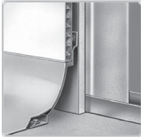
FIGURE 12 The wall system used in the facility incorporates a monolithic sheet vinyl flooring junction between floor and wall face. Note the coving run up the wall around the edges to provide a smooth surface for cleaning. (Courtesy of Portafab.)
