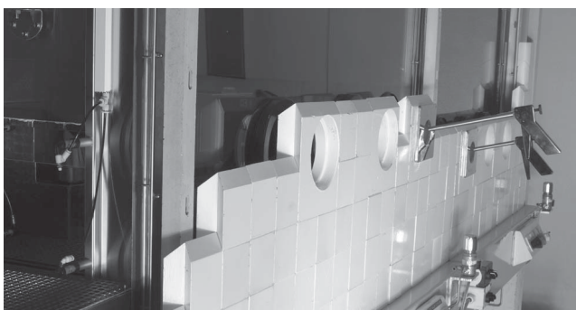
FIGURE 3 Lead bricks are interlocked when they are stacked on top of each other. (Photo courtesy of Institute for Energy Technology.)
