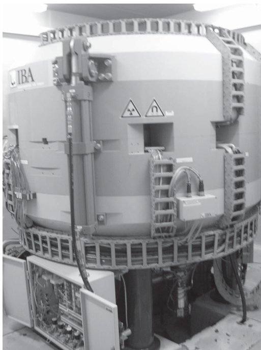
FIGURE 5 Small (less than 2 m in diameter) dual-beam negative ion cyclotron capable of easily producing multicurie amounts of ^{18}\text{F} and ^{11}\text{C} . (Photo courtesy of PET-CUN Center, University of Navarra.)
