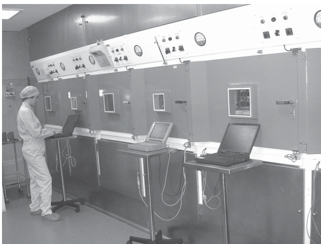
FIGURE 8 Production laboratory for PET radiopharmaceuticals. The 10-cm lead shielded hot cells contain computer-controlled automated synthesis modules. (Photo courtesy of PET-CUN Center, University of Navarra.)
