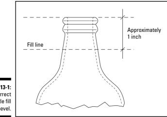
Figure 13-1: Correct bottle fill level.
