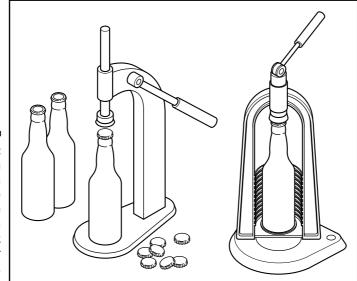
Figure 2-3: You can attach a bench-type bottle capper to a work surface for easy use.
