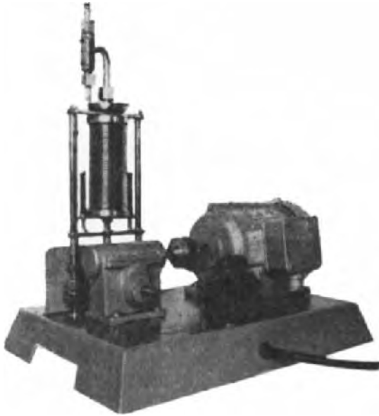
Fig. 400 Electric spring bellows metering pump for liquids and gases
