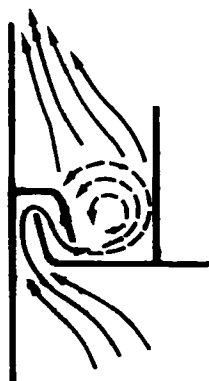
Fig. 264a) Vapour path through collision plates
