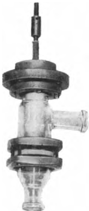
Fig. 247 Precision valve of glass with PTF spindle for the control of liquid and gas flow (face and tube diameter d = 4 and 7 mm)
