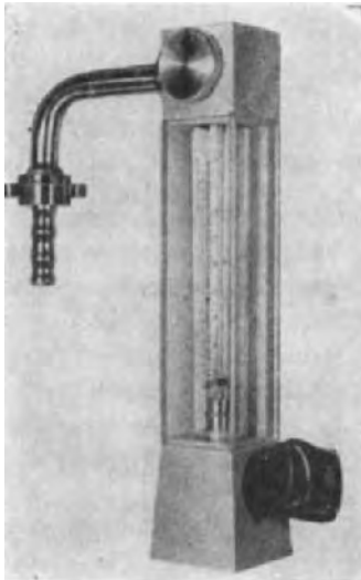
Fig. 395 Laboratory flow meter, type SW 16.1 Measuring range I: 0.5 to 3.0 l/min; range II: 3.0 to 12.0 l/min
