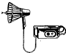
Fig. 191 High-frequency leak detector with brush electrode and ratio shielding
