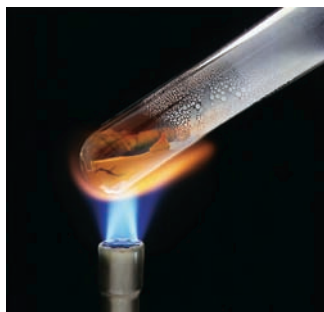
When heated, HgO decomposes to give Hg and O 2 .
