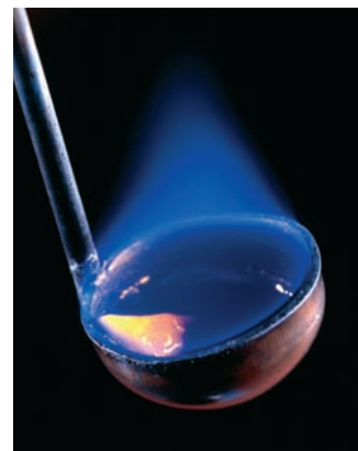
Sulfur burning in air to form \text{SO}_2 .
