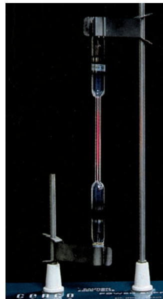
Figure 7.6 Color emitted by hydrogen atoms in a discharge tube. The color observed results from the combination of the colors emitted in the visible spectrum.
