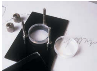
A salt plate used for IR spectroscopy. These plates are moisture sensitive and must be stored in a moisture-free environment.
