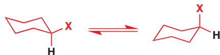
ring inversion of a monosubstituted cyclohexane notice that the hydrogen atom shown changes from axial to equatorial
