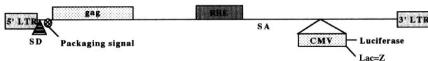
Figure 5 The transfer vector incorporates both the 5' and 3' LTR sequences removed from the original provirus when making the packaging construct. The promoter before the gag sequences has been removed along with most of the original envelope proteins. The gag gene is truncated and out of frame, and the internal CMV promoter is used to drive expression of a reporter gene such as lac-Z or luciferase. The RRE and splice acceptor site (SA) are indicated.
