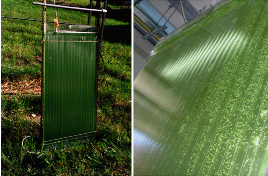
Fig. 5 Thin flat plate air lift photobioreactors (LNEG, Portugal)
