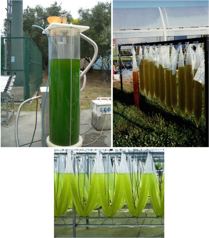
Fig. 6 Vertical column photobioreactors (LNEG, Portugal)
