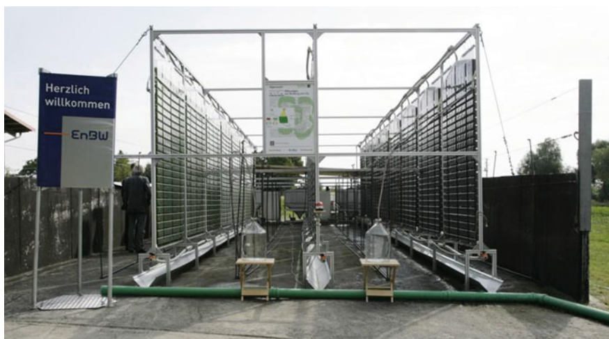
Fig. 9 Flat panel airlift reactor (Subitec) ( http://www.subitec.com ). Photo courtesy of Subitec
