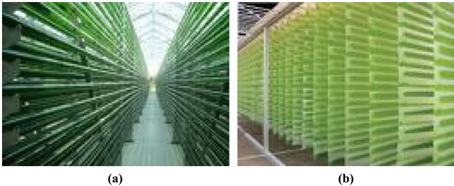
Figure 4.3 (a) Tubular and (b) vertical photobioreactors
