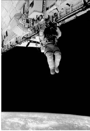
Figure 13-3. Floating inverted in Shuttle payload bay can cause EVA Height Vertigo (NASA photo)
