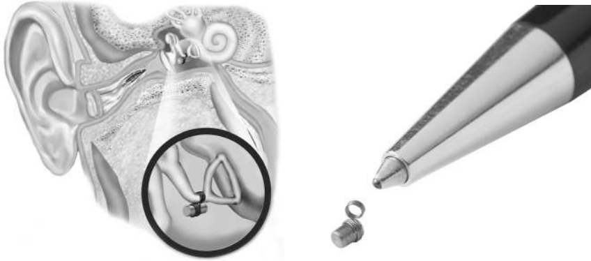
Figure 10.6 Direct System MEIHD (SOUNDTEC, Inc.; Oklahoma City, OK). This semi-implantable electromagnetic device is shown on the left; the sound processor and electromagnetic coil are worn in the ear canal. The magnet implant portion is surgically placed through the ear canal and attached around the incudostapedial joint. The implant portion (right) is a permanent magnet hermetically sealed in a titanium canister.
