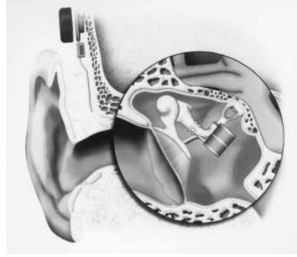
Figure 10.7 Vibrant Soundbridge MEIHD (Symphonix Devices, Inc.; San Jose, CA). This semi-implantable electromagnetic device is shown on the left, where a transducer (magnet and encircling coil) is attached to the incus. The internal receiver demodulates an radiofrequency signal containing frequency and amplitude information. The middle ear placement is depicted on the right; the hardwired, hermetically sealed transducer is attached to the incus.
