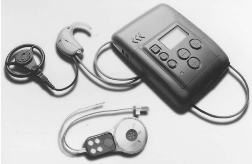
Figure 10.11 Auditory Brainstem Implant (Cochlear Corp.; Englewood, CO). The wearable speech processor (upper) has an ear-level microphone and associated transmitting antenna, and the magnet for attachment contains the batteries and sound processing circuitry. The implant portion (below) is comparable to a cochlear implant with a ball and ground electrode but with a flat surface array of electrodes at the end of the second cable that is placed on the medullary surface, over the cochlear nucleus. The implant also contains a receiving antenna, attaching magnet, and demodulating circuit.
