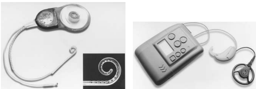
Figure 10.9 Nucleus 24 Contour CI (Cochlear Corp.; Englewood, CO). The ear-level sound processor (right) contains a microphone, battery, sound processing circuitry, and transmitting antenna with magnet in its center for attachment to the head of a patient. The implant (left) contains a receiving antenna, demodulating circuit, ground (ball) electrode, and semibanded electrode array (22) at the end of the second cable.
