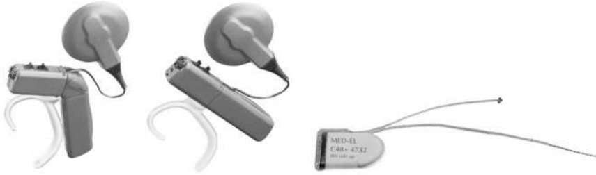
Figure 10.10 COMBI-40+ CI (MED-EL Corp.; Innsbruck, Austria). The ear-level sound processor (upper) contains a microphone, battery, sound processing circuitry with ear hook for attachment to the ear, and transmitting antenna with magnet in its center for attachment to head of a patient. The implant (below) contains a receiving antenna, demodulating circuit, ground (ball) electrode, and split electrode array (12 pairs) at the end of the second cable.
