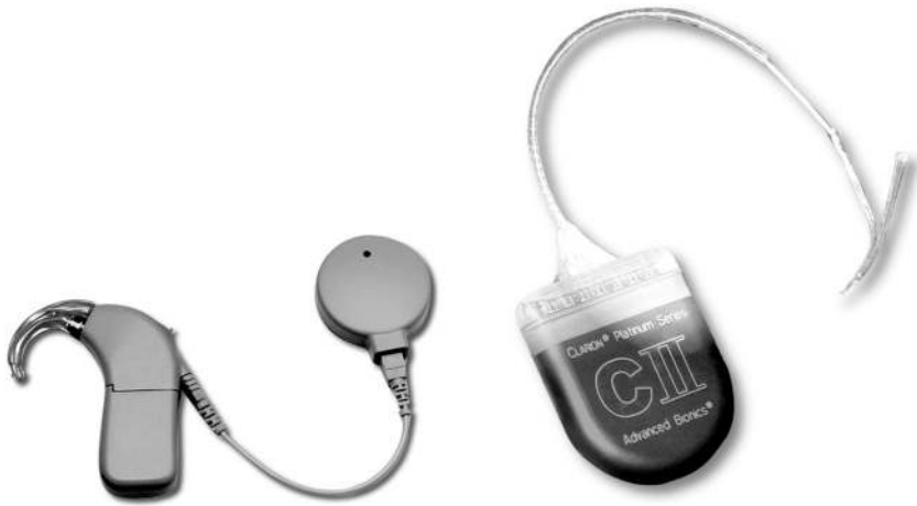
Figure 10.8 Clarion II Bionic Ear system CI (Advanced Bionics, Inc.; Sylmar, CA). The ear-level sound processor (left) contains microphone, battery, sound processing circuitry, transmitting antenna, and magnet for attachment to the head of a patient. The implant (right) contains a receiving antenna, demodulating circuit, and planar contact electrode array (31) at the end of the cable. Both Clarion and Nucleus electrode arrays are curved to fit inside the cochlear canal.
