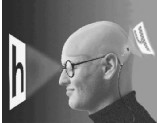
Figure 11.8 Artist's concept of a cortically based visual neuroprosthesis. A small camera, located in the bridge of a pair of glasses, encodes the visual scene. This signal then drives a small array of electrodes implanted into primary visual cortex. The signal-processing electronics, not shown, convert the video signal into controlled current pulses on each of the electrodes, resulting in the percept of the same pattern seen by the camera.
