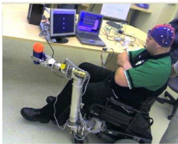
Fig. 5. A user controlling the WMRA by choosing characters from the BCI display
