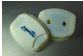
Fig. 7. Custom NIR sensor for verbal cognitive activity detection and analysis
