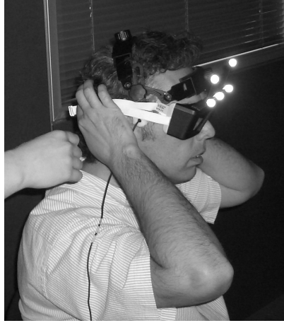
Fig. 2. User with TCD probes and shutter glasses for visualizing VE with stereoscopy
