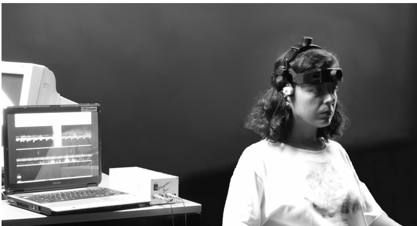
Fig. 1. Subject with TCD probes placed in their correct location with the help of a probe holder
