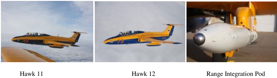
Fig. 1. OPL's Instrumented L-29 Fighter Jet Trainer Aircraft
