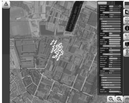
Fig. 4. Cerberus screen appearance. The application displays the relevant parameters of each firemen, such as location (represented by helmets), reported incidents, fire development, and risk of collapse.
