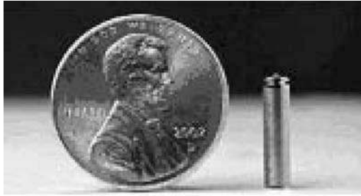
FIGURE 18.2 Quallion battery for the BPB.
