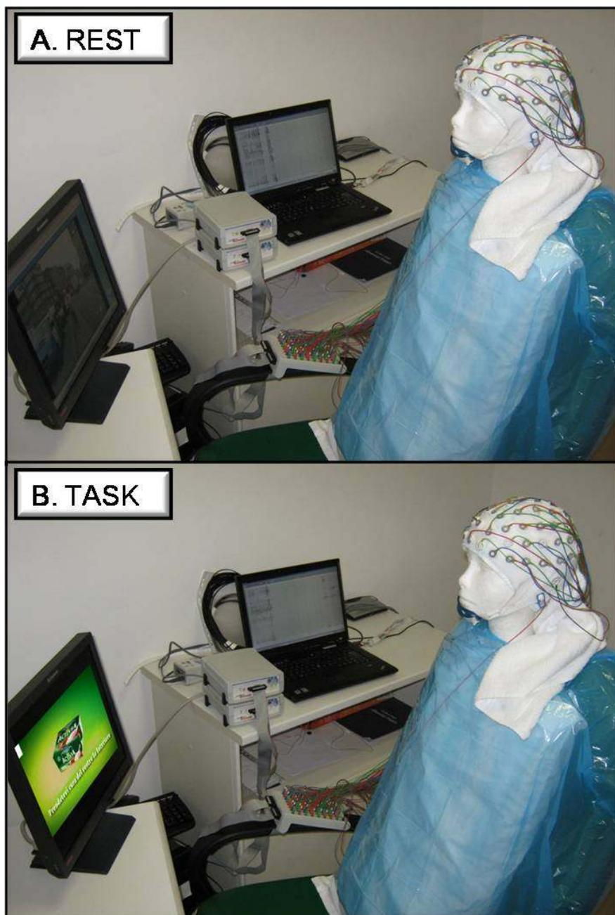
**Fig. 5** Figure presents the experimental setup employed for the electrical recordings. In this picture we may see the mannequin in both experimental conditions. Panel A shows the mannequin in front of the screen while the documentary is playing (REST); panel B shows the mannequin while a commercial advertisement is playing on the screen.
