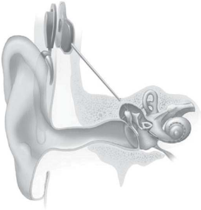
Figure 10.2. Schematic diagram of a cochlear implant. The external components consist of a microphone, a sound processor, and a transmitter of power and processed signals. The internal components consist of a receiver and stimulator, along with an array of electrodes that can be seen wound up within the cochlea in the figure. (Image: Creative Commons).
