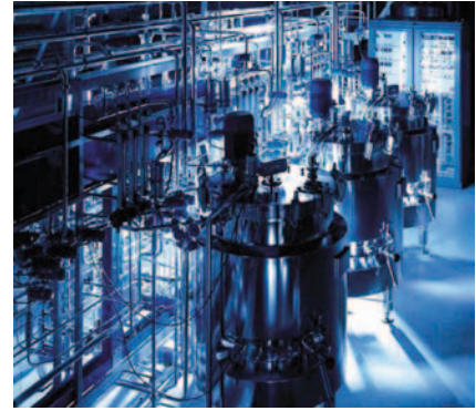
Figure 4–50 Biotechnology companies produce mass quantities of useful proteins. Shown in this photograph are the fermenters used to grow the cells needed for such large-scale protein production. (Courtesy of Bioengineering AG, Switzerland.)
