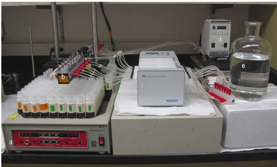
Fig. 4 Automated continuous flow perfusion system showing (a) fraction collector with collection vials in movable racks. Water-jacketed support blocks (b) holding perfusion cells are connected by tubing to the peristaltic pump (c) that delivers collection fluid from a reservoir (e). The temperature of the cells is controlled by the water pumped through the support blocks from the circulating water bath (d)
