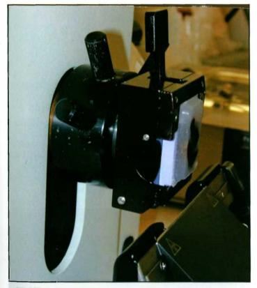
[i3.18] The block holder shaft is correctly positioned.
