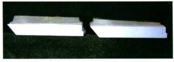
**[i3.9]** The entire face of the block was not parallel to the blade, so that ribboning was very uneven, and a major part of one side of the block has been cut away.
