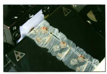
**[i3.22]** The results of a major nick, or defect, in the blade edge can be seen in this paraffin ribbon. This defect possibly resulted from improper handling of the forceps used in sectioning. Any metallic object that is allowed to come into contact with the blade edge can damage the edge and cause this type of artifact.
