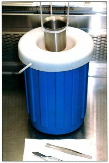
**[i13.5]** The equipment for freezing a specimen is shown. The small beaker contains isopentane; it will be lowered into the container of liquid nitrogen.
