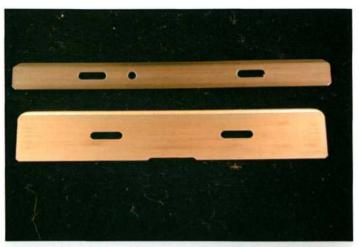
**[i3.25]** High- and low-profile blades are shown; the high-profile blade (bottom) is commonly used for frozen sectioning.
