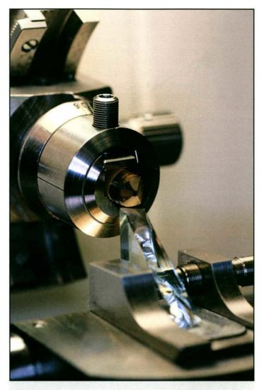
[i14.7] Glass knives have been used for many years to cut 0.5-µm sections for microscopic examination.
