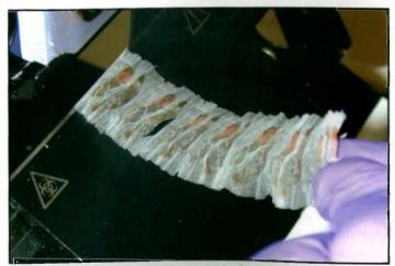
**[i3.21]** Compressed sections, as seen in this figure, may result from a dull blade, too little blade tilt, paraffin accumulation on the blade, and cutting too rapidly.
