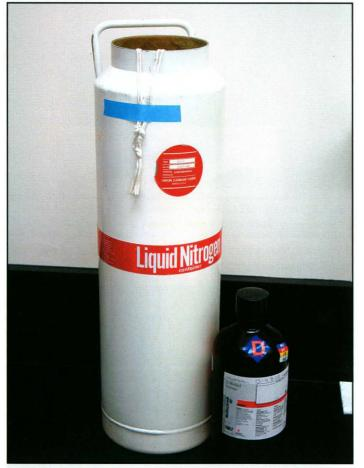
**[i13.8]** The beaker of isopentane can be suspended in a Union Carbide liquid nitrogen container. If the string is threaded through a hole made in the cork before freezing, the frozen specimen can be left suspended in liquid nitrogen until ready to section, or after sectioning until ready for long-term storage. If necessary, the string can be taped to the outside of the container for easy retrieval.
