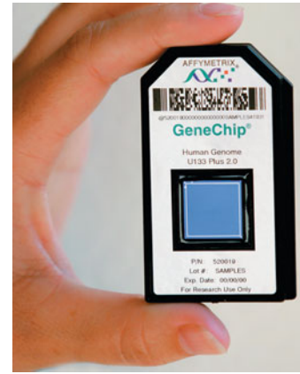
FIGURE 22-18 A commercially available DNA microarray, called a GeneChip, marketed by Affymetrix, Inc. This microarray can be used to analyze expression for approximately 50,000 RNA transcripts. It contains 22 different probes for each transcript and allows scientists to simultaneously assess the expression levels of most of the genes in the human genome.
