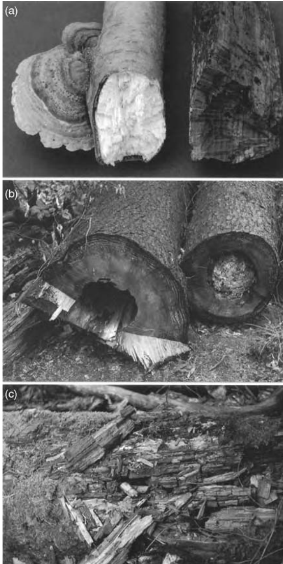
Fig 19.12 Wood rot symptoms. (a) White-rot of beech caused by Trametes hirsuta (left). Note the bleached appearance of the branch interior at the broken surface. Beech wood attacked by a brown-rot is also shown for comparison (right). (b) Trunk segments of Picea abies attacked by Fomitopsis pinicola . The brown-rot had caused a hollowing of the standing tree prior to felling. (c) Log of Picea abies colonized by Fomitopsis pinicola , showing brown rot symptoms. The wood has cracked into cube-like fragments which are easily ground into a powder.
